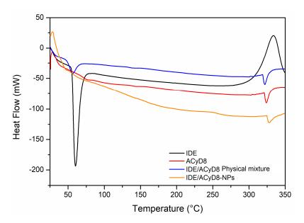
**Figure 12.** DSC traces of IDE/ACyD8-NPs (sample C), pure IDE and ACyD8, and the physical mixture.
