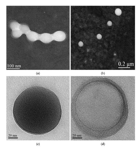
**Figure 10.** STEM images of lyophilized IDE/ACyD8-NPs before (**a**) and after redispersion (**b**). The NPs observed at higher magnification showed both matrix structure (**c**) and nanoreservoir structure (**d**).
