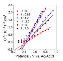
**Figure 8.** Mott-Schottky plots of (black)  $WO_3-0$ , (pink)  $WO_3-0.62$ , (blue)  $WO_3-1.2$ , (red)  $WO_3-2.5$ , (wine)  $WO_3-5$ , and (navy)  $WO_3-7.5$  electrodes in a 0.1 M phosphate buffer solution of pH 6.0. frequency, 0.1 Hz; amplitude potential, 10 mV.
