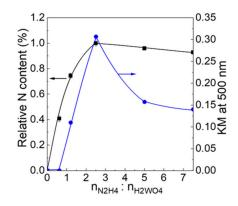
**Figure 7.** Relationship between the relative contents of N and  $n_{H2WO4}$ : $n_{N2H4}$  ratio. The relative N contents were measured in EDS data and normalized by the highest contents for  $n_{H2WO4}$ : $n_{N2H4}$  of 1:2.5.
