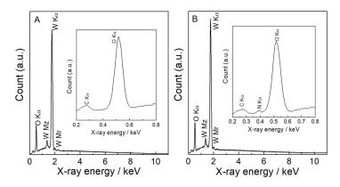
**Figure 2.** The EDS data of (**A**)  $WO_3 - 0$  and (**B**)  $WO_3 - 2.5$  in the range of 0–11 keV. (Insert) The magnified EDS data of  $WO_3 - 0$  and  $WO_3 - 2.5$  in the range of 0.2–0.8 keV, respectively.
