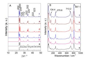
**Figure 3.** (**A**) XRD patterns and (**B**) Raman spectra of (a) WO<sub>3</sub>-0, (b) WO<sub>3</sub>-0.62, (c) WO<sub>3</sub>-1.2, (d) WO<sub>3</sub>-2.5, (e) WO<sub>3</sub>-5, and (f) WO<sub>3</sub>-7.5, respectively.
