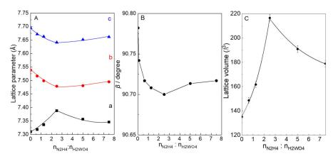
**Figure 4.** (**A**) Plots of lattice parameters of (a), (b), and (c) versus the addition of N<sub>2</sub>H<sub>4</sub>. (**B**) Plots of  $\beta$  versus the addition of N<sub>2</sub>H<sub>4</sub>, and (**C**) Lattice volumes of N<sub>2</sub>-intercalated WO<sub>3</sub> samples prepared with addition of N<sub>2</sub>H<sub>4</sub>. The lattice volume (V) was calculated according to equation: V = *abc*(sin $\beta$ ),  $\beta$  is the angle between a and c.
