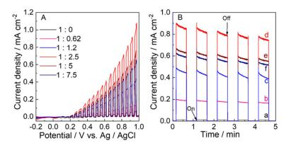
**Figure 9.** (**A**) Linear sweep voltammograms (LSV), and (**B**) Time course of the photocurrent at 0.68 V vs. Ag/AgCl (1.23 V vs. RHE) of the (a) WO<sub>3</sub>-0, (b) WO<sub>3</sub>-0.62, (c) WO<sub>3</sub>-1.2, (d) WO<sub>3</sub>-2.5, (e) WO<sub>3</sub>-5, and (f) WO<sub>3</sub>-7.5 electrodes with visible-light irradiation chopped in a 0.1 M phosphate buffer solution of pH 6.0 with visible-light irradiation ( $\lambda > 450$  nm, 100 mW cm<sup>-2</sup>).
