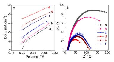
**Figure 12.** (A) Tafel plots and (B) Nyquist plots of (a)  $WO_3-0$ , (b)  $WO_3-0.62$ , (c)  $WO_3-1.2$ , (d)  $WO_3-2.5$ , (e)  $WO_3-5$ , and (f)  $WO_3-7.5$  electrodes for photoelectrocatalytic water oxidation in a 0.1 M phosphate buffer solution (pH = 6).
