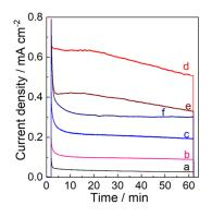
**Figure 11.** Photocurrent density versus time profiles during PEC water oxidation in a 0.1m phosphate buffer solution of pH 6.0 at 0.68 V vs. Ag/AgCl (1.23 V vs. RHE) upon visible-light irradiation ( $\lambda > 450 \text{ nm}$ , 100 mWcm<sup>-2</sup>) using (a) WO<sub>3</sub>-0, (b) WO<sub>3</sub>-0.62, (c) WO<sub>3</sub>-1.2, (d) WO<sub>3</sub>-2.5, (e) WO<sub>3</sub>-5, and (f) WO<sub>3</sub>-7.5 electrodes.
