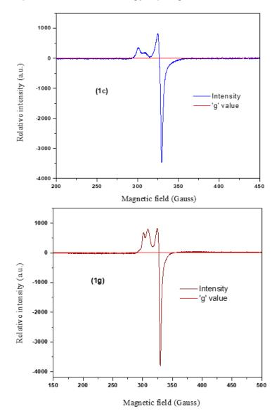
Figure 3. X-band EPR spectrum of complex [Cu(L)(phen)] 1c and [Cu(L)(bpy)] 1g at room temperature.
