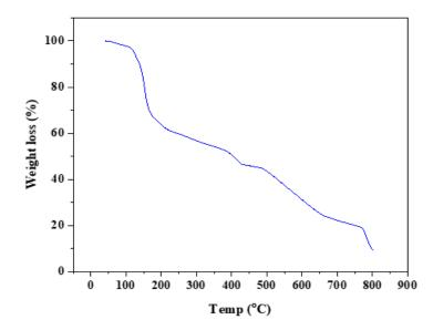
**Figure 2.** TGA curve of [Cu(L)(bpy)] **1g** complex.
