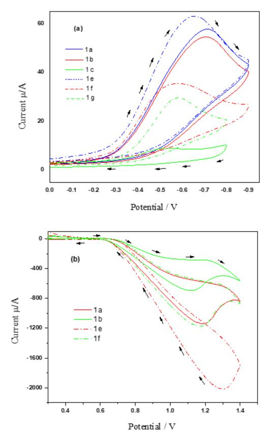
**Figure 5.** Cyclic voltammograms of metal(II) complexes **1a–h**. (**a**) Reduction process at cathodic region. (**b**) Oxidation process at anodic region in DMF containing 0.1M of tetra(n–butyl)ammoniumperchlorate. The scan rate applied was 100 mVs<sup>-1</sup>.
