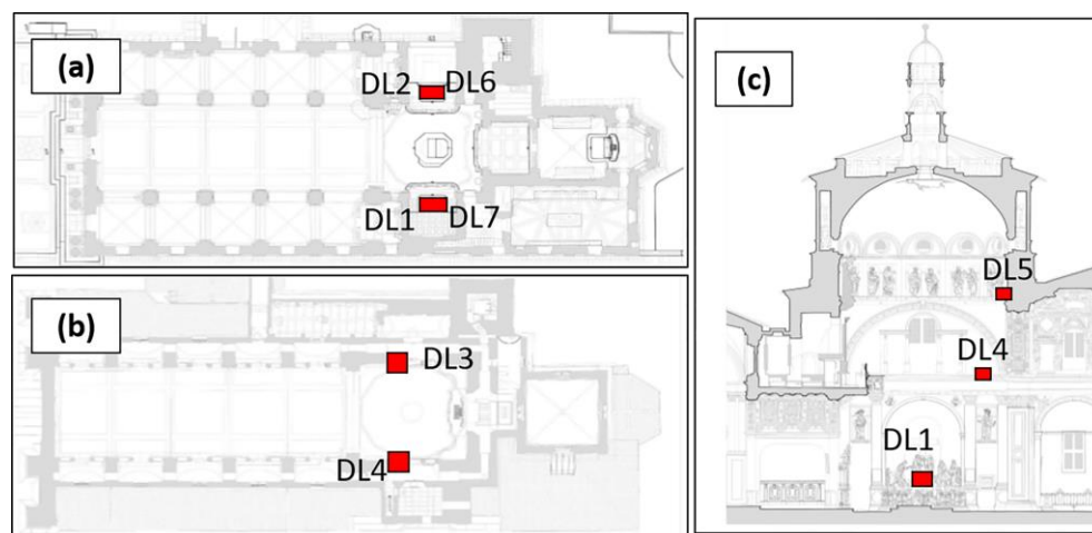
Figure 10. The floor plans and sections of the sanctuary showing the placement of the dataloggers: (a) Ground floor plan, (b) first floor plan, (c) right-side section ( Deposition ).
