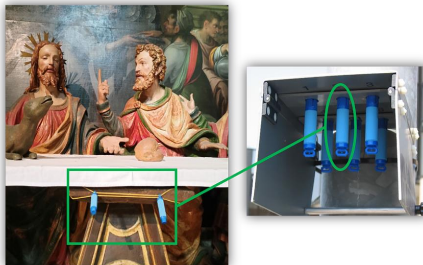
Figure 13. Diffusive passive samplers positioned in one of the main chapels close to the sculptural group of the Last Supper .
