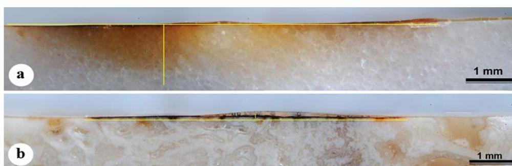
**Figure 3.** Artificially stained samples. Cross sections images acquired in reflected light (10×) of Carrara marble (a) and Travertine (b) stained outdoors for two seasons (spring and summer).
