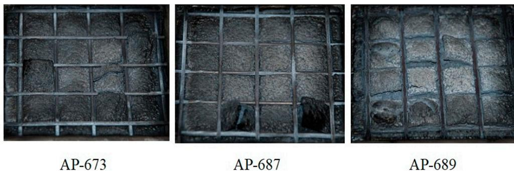
**Figure 16.** Photographs of the residua after cone calorimeter test of AP-673, AP-678 and AP-689.
