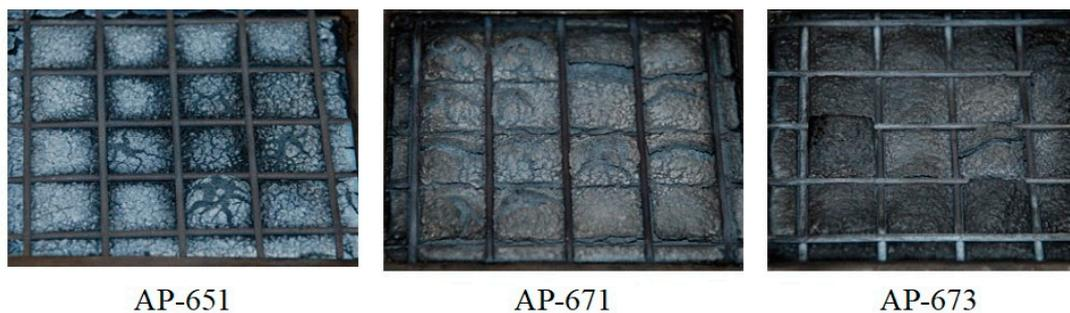
**Figure 6.** Photographs of the residua after cone calorimeter test of AP-651, AP-671 and AP-673.
