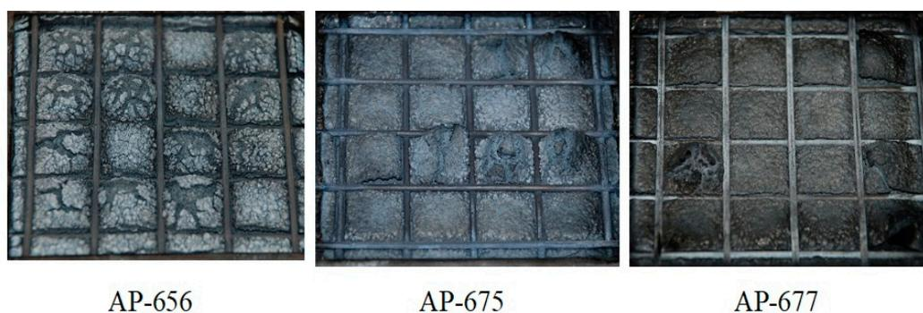
Figure 11. Photographs of the residua after cone calorimeter test of AP-656, AP-675 and AP-677.
