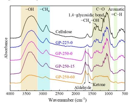
Figure 4. The FTIR spectrum of raw and GP-torrefied cellulose.
