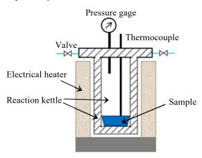
Figure 8. The schematic diagram of the GP torrefaction system.
