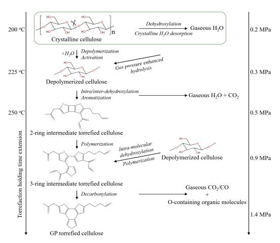
Figure 7. The schematic diagram of the GP torrefaction mechanism of cellulose.
