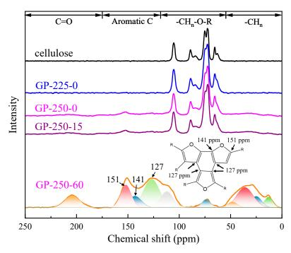
**Figure 5.** The <sup>13</sup>C NMR of the raw and torrefied cellulose.
