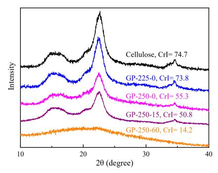
**Figure 3.** The XRD patterns of raw and GP-torrefied cellulose.
