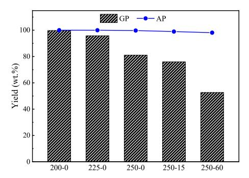
**Figure 1.** Mass yields of cellulose torrefied by GP and AP torrefactions.
