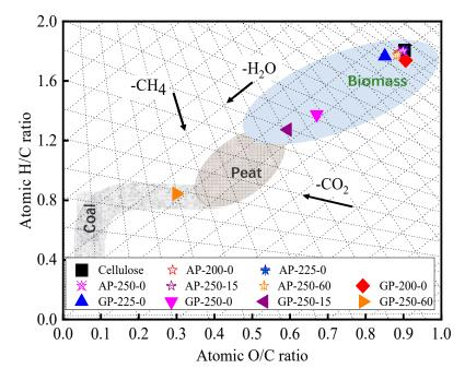
**Figure 2.** Van Krevelen diagram for raw and torrefied cellulose.
