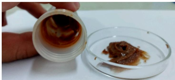
**Figure 10.** Grease obtained from lithium anacardate and paraffin oil.
