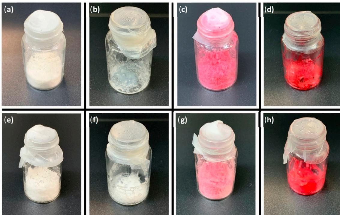
**Figure 6.** Representative images of lyophilized VB<sub>12</sub> lipid vesicles: (a) empty liposome with lactose, (b) empty liposome with sorbitol, (c) VB<sub>12</sub>-loaded liposome with lactose, (d) VB<sub>12</sub>-loaded liposome with sorbitol, (e) empty transfersome with lactose, (f) empty transfersome with sorbitol, (g) VB<sub>12</sub>-loaded transfersome with lactose, and (h) VB<sub>12</sub>-loaded transfersome with sorbitol. Reprinted from [107].
