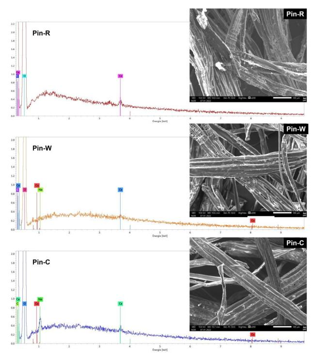
**Figure 1.** Comparison of scanning electron microscopy images and elemental analysis spectra by energy-dispersive spectroscopy of raw pine (Pin-R), washed pine (Pin-W) and activated pine (Pin-C) materials.
