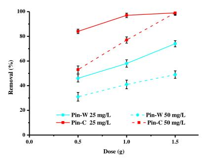
**Figure 7.** Effect of the mass of adsorbent used on copper abatement (expressed in % of removed pollutant) by washed (Pin-W) and activated (Pin-C) pine materials at two different concentrations, 25 and 50 mg/L (other conditions: volume of solution = 100 mL; contact time = 120 min; T = 22  $\pm$  1 °C; pH<sub>i</sub> = 5.2–5.4  $\pm$  0.1; agitation = 250 rpm; n = 3).
