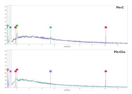
**Figure 12.** EDS spectra of Na<sub>2</sub>CO<sub>3</sub> activated maritime pine samples before (Pin-C) and after adsorption (Pin-CCu).
