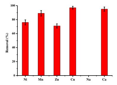
**Figure 10.** Comparison between adsorption capacities (expressed in % of removed pollutant) of activated pine material towards several cations present in monocontaminated solution at a concentration of 25 m/L (other conditions: volume of solution = 100 mL; mass of material = 1 g; contact time = 120 min;  $T = 22 \pm 1$  °C; stirring = 250 rpm;  $pH_i = 5.4-5.9 \pm 0.1$ ; n = 5).
