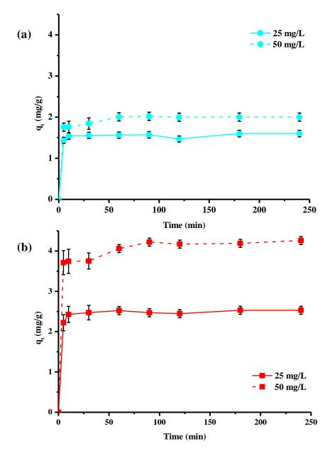
**Figure 3.** Kinetics of adsorption of copper ions by washed Pin-W (a) and activated Pin-C (b) pine materials at two different concentrations, 25 and 50 mg/L (other conditions: solution volume = 100 mL; mass of material = 1 g; T =  $22 \pm 1$  °C; pH<sub>i</sub> = 5.2– $5.4 \pm 0.1$ ; stirring = 250 rpm; n = 3).
