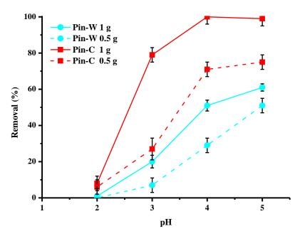
**Figure 8.** Effect of the initial pH of the solution on copper abatement (expressed in % of removed pollutant) by washed (Pin-W) and activated (Pin-C) pine materials at two different masses, 0.5 and 1 g (other conditions: volume of solution = 100 mL; [Cu] = 25 mg/L; contact time = 120 min;  $T = 22 \pm 1$  °C; stirring = 250 rpm; n = 3).
