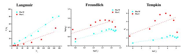
**Figure 6.** Representations of adsorption isotherms of experimental results modelled by the Langmuir, Freundlich and Temkin equations.
