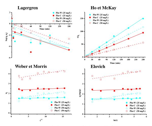
**Figure 4.** Graphical representations of the kinetic models of Lagergren, Ho and McKay, Weber and Morris, and Elovich for Pin-W washed pine and Pin-C activated pine materials at two different concentrations, 25 and 50 mg/L.
