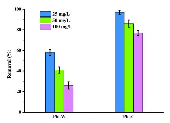
**Figure 2.** Comparison of copper abatements (expressed in % of removed pollutant) obtained on two pine materials, washed (Pin-W) and activated (Pin-C), at three initial concentrations of copper (other conditions: volume of solution = 100 mL; mass of material = 1 g; contact time = 120 min;  $T = 22 \pm 1$  °C;  $pH_i = 5.1-5.4 \pm 0.1$ ; agitation = 250 rpm; n = 5).
