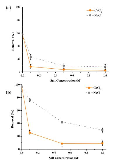
**Figure 9.** Effect of presence of NaCl and CaCl<sub>2</sub> in the solution on copper abatement (expressed in % of removed pollutant) by Pin-W (**a**) and activated Pin-C (**b**) pine materials (other conditions: volume of solution = 100 mL; mass of material = 1 g; [Cu] = 25 mg/L; [Na<sup>+</sup>] = [Ca<sup>2+</sup>] = 0.1, 0.5 and 1 mol/L; contact time = 120 min;  $T = 22 \pm 1$  °C; stirring = 250 rpm;  $pH = 5.4 \pm 0.1$ ; n = 3).
