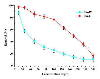
**Figure 5.** Effect of the initial copper concentration on the purification performance (expressed in % of removed copper) of washed (Pin-W) and activated (Pin-C) pine materials (other conditions: volume of solution = 100 mL; mass of material = 1 g; contact time = 120 min; T = 22  $\pm$  1 °C; pH<sub>i</sub> = 4.7–5.6  $\pm$  0.1; stirring = 250 rpm; n = 3).
