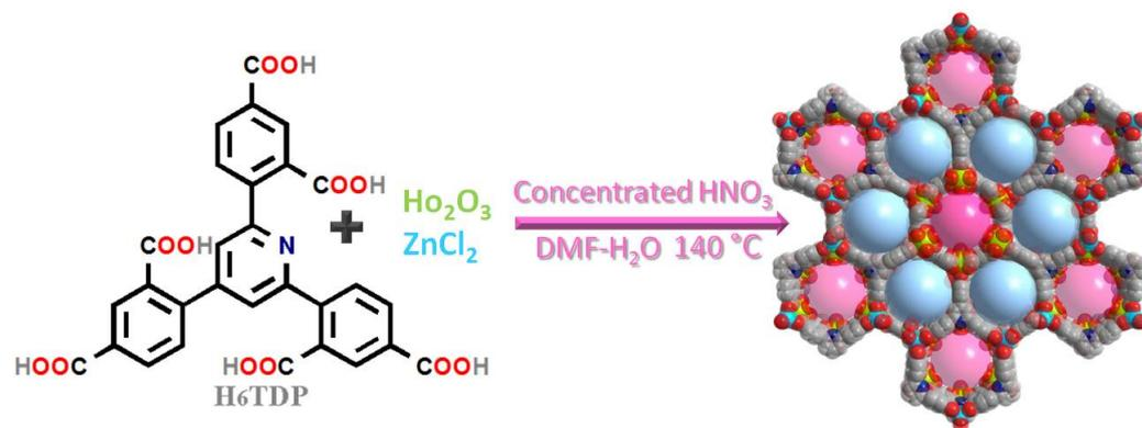
**Scheme 1.** The preparation process of the heterometallic ZnHoMOF.
