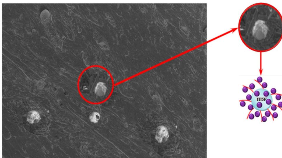
**Figure 2.** SEM microphotograph of vulcanized stock 10MUV:5MSF (magnification  $\times 10,000$ ).
