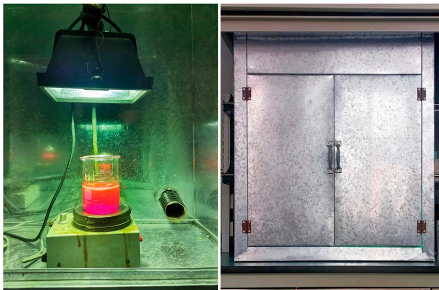
**Figure 14.** Self-made photocatalytic experimental apparatus.
