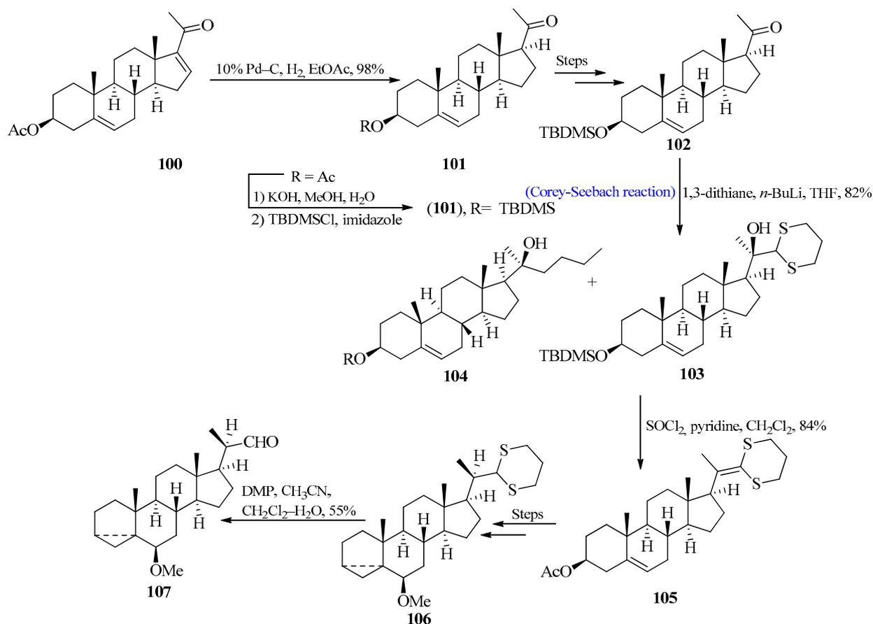
**Scheme 16.** Synthesis of cholanic acid derivatives **107** by utilizing Corey-Seebach approach.
