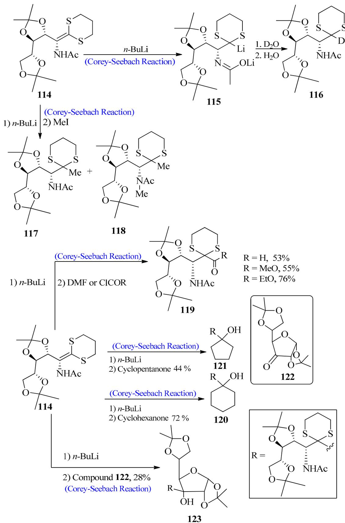
Scheme 18. Synthesis of D-glucosamine derivatives 123 via Corey-Seebach approach.
