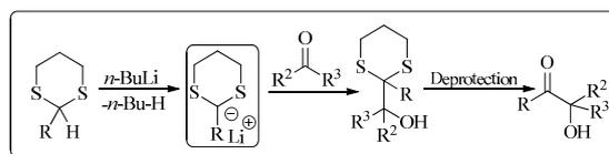
**Figure 1.** A typical Corey-Seebach reaction.
