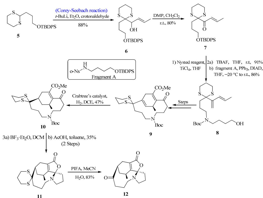
**Scheme 1.** Synthesis of lycoplanine A **12** isomer via Corey-Seebach reagent.
