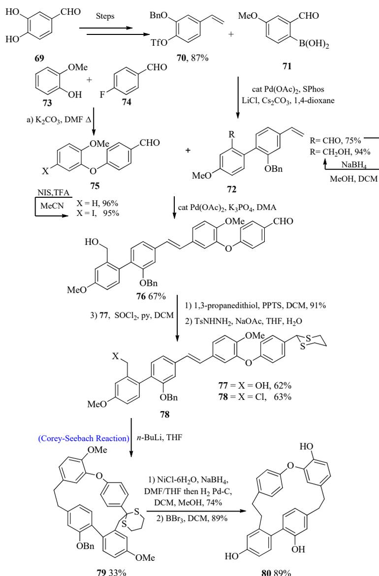
**Scheme 11.** Synthesis of riccardin C **80** via Corey-Seebach reaction.
