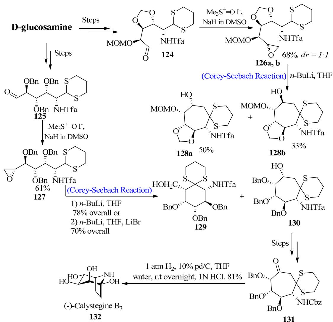
**Scheme 19.** Synthesis of (–)-calystegine B<sub>3</sub> **132** by utilizing Corey-Seebach reaction.
