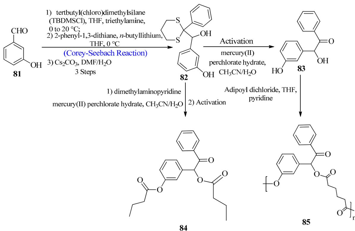
**Scheme 12.** Synthesis of benzoin-derived diol linkers **84** and **85**.
