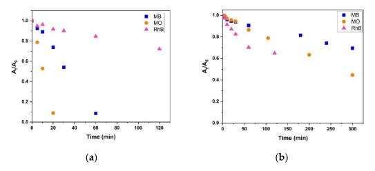
**Figure 6.** Plot of  $A_t/A_0$  vs. time for decolorization of 3 dyes (MB, MO, and RhB) using (**a**) [MnL<sub>2</sub>Cl] and (**b**) [FeL<sub>2</sub>Cl] as catalysts. [Note: The time = 0 initial points for all three dyes are congruent, as the time = 0 point is defined as 1.0 in the ratio  $A_t/A_0$  for all three dyes. Individual plots of each dye are available in the supplementary information.].
