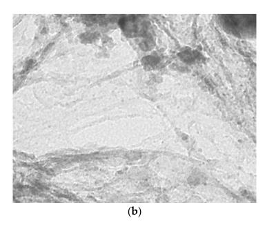
**Figure 4.** TEM images of calcined 10%Cu/SiO<sub>2</sub> catalysts obtained by microwave-assisted synthesis (a) and DPU method (b).
