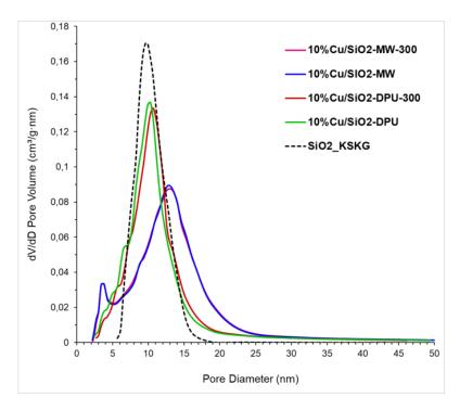
**Figure 3.** Pore size distributions of the 10%Cu/SiO<sub>2</sub> catalysts.
