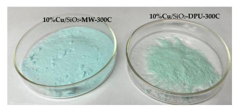
**Figure 5.** Photos of calcined samples 10%Cu/SiO<sub>2</sub> obtained by microwave (MW) and thermal (DPU) hydrolysis of urea.
