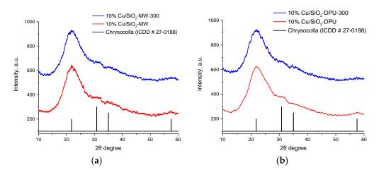
**Figure 1.** XRD profiles for dry and calcined 10%Cu/SiO<sub>2</sub> samples obtained by microwave synthesis (a) and DPU method (b).
