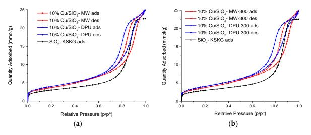
**Figure 2.**  $N_2$  adsorption–desorption isotherms of prepared catalysts: dried samples (**a**) and calcined at 300  $^{\circ}$ C samples (**b**).
