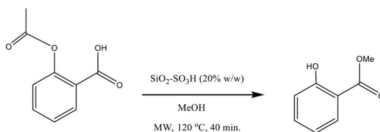
**Figure 1.** Reactions of the conversion of ASA into MS. The synthesis proceeds via the tandem transesterification–esterification reaction catalyzed by SiO<sub>2</sub>–SO<sub>3</sub>H.
