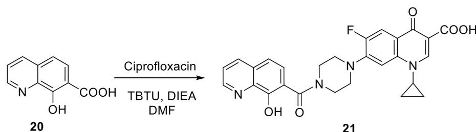
**Scheme 7.** Preparation of 8-hydroxyquinoline-ciprofloxacin hybrid 21.
