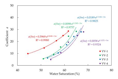
Figure 7. The relationship between the coefficient *a* in Formula (7) and water saturation.
