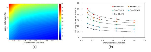
**Figure 3.** The relationship between viscosity retention rate of polymer solution, dimensionless distance and water saturation in the experiment VV-1 in which the polymer concentration is 500 mg/L. (a) Contour map of viscosity retention rate; and (b) scatter plot of viscosity retention rate.
