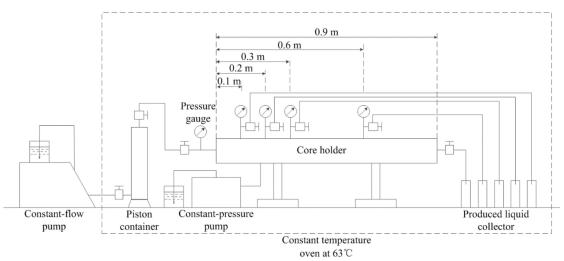
Figure 2. Experiment-process diagram.
