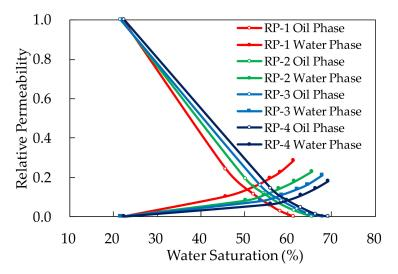
**Figure 8.** The relative permeability curves of polymer flooding calculated by the improved J.B.N. method.
