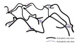
Figure 1. Three-dimensional schematic diagram of interactions of hydrophobically associating polymers.
