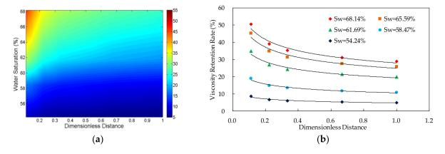
**Figure 6.** The relationship between viscosity retention rate of polymer solution, dimensionless distance and water saturation in the experiment VV-4 in which the polymer concentration is 2000 mg/L. (a) Contour map of viscosity retention rate; and (b) scatter plot of viscosity retention rate.
