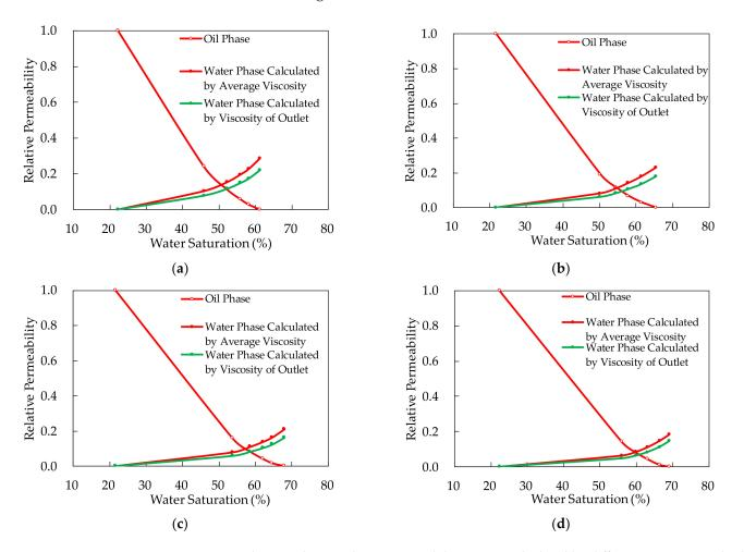
Polymer solution relative permeability curves calculated by different viscosity methods were shown in Figure 9.
