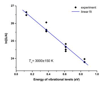
Figure 4. Boltzmann plot estimating the vibrational temperature of the nitrogen molecules.
