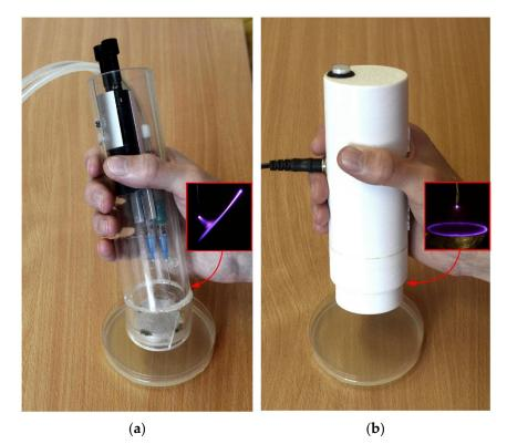
**Figure 1.** The developed sources of NTP: (**a**) source of NTP based on the cometary discharge; (**b**) source of NTP based on the point-to-ring discharge.
