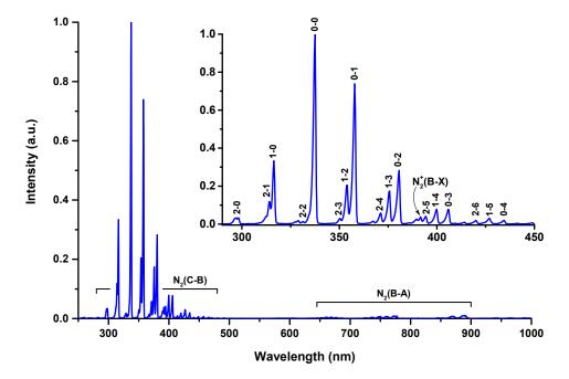
**Figure 3.** Typical time-integrated emission spectrum of the cometary/point-to-ring discharge. The inset shows the short-wavelength region of the emission spectrum.
