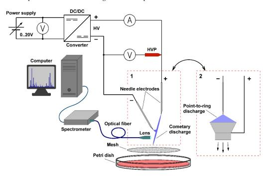
**Figure 7.** Experimental setup: 1—point-to-point electrode configuration for the cometary discharge, 2—point-to-ring electrode configuration for the corona discharge.
