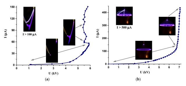
**Figure 2.** The volt–ampere characteristics and relevant images of the cometary discharge (**a**) and the point-to-ring discharge (**b**).
