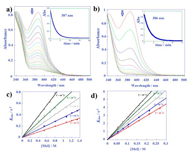
**Figure 4.** The changes in the UV-visible spectra of (**a**) **1a** and (**b**) **1c** with MeI in acetone at 25  $^{\circ}$ C (inset is the variation of absorbance at a corresponding wavelength over time). Plots of the first-order rate constants ( $k_{\rm obs}/{\rm s}^{-1}$ ) for the reactions of (**c**) **1a** and (**d**) **1c** with MeI in acetone at different temperature conditions versus MeI concentration.
