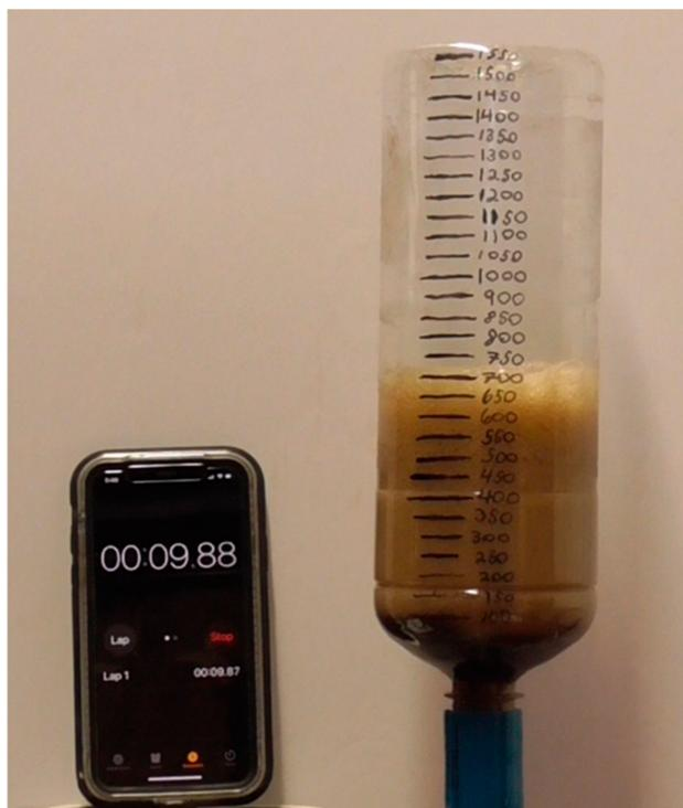
**Figure 7.** Image of home-built foam collector pictured 4.88 s after dropping a single Mentos candy into a sample prepared from 500 mL of Diet Coke at 20 °C.
