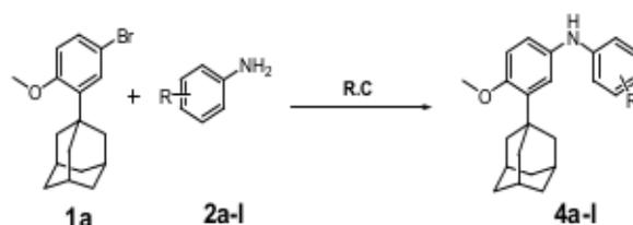
**Scheme 1.** Reported scheme to show the coupling of adamantane bromides with various aromatic amines to obtain adamantanyl-tethered-biphenyl amines (ATBAs). R.C: Reaction conditions; PS-Co (BBZN)Cl<sub>2</sub> (12 mol %); CS<sub>2</sub>CO<sub>3</sub> (3 Eq); BINAP (15 mol %); 1,4-dioxane (5 mL); N<sub>2</sub> atmosphere 10 h; 100 °C.
