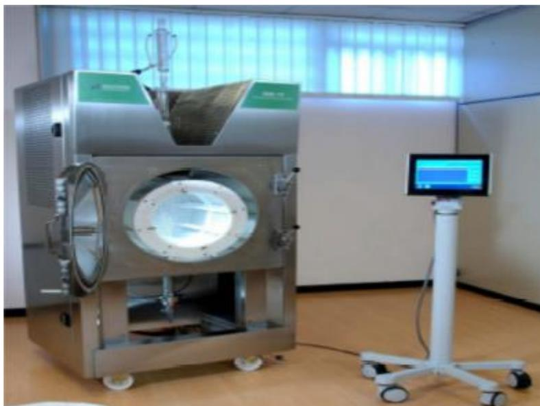
**Figure 5.** The setup of the industrial scale microwave extractor model MAC–75/Milestone Technologies.
