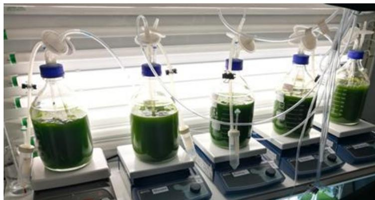
Figure 8. Photobioreactor for the batch accumulation test.
