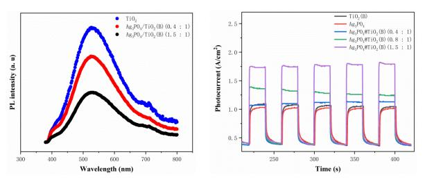
Figure 7. PL and photocurrent spectra of synthesized samples.
