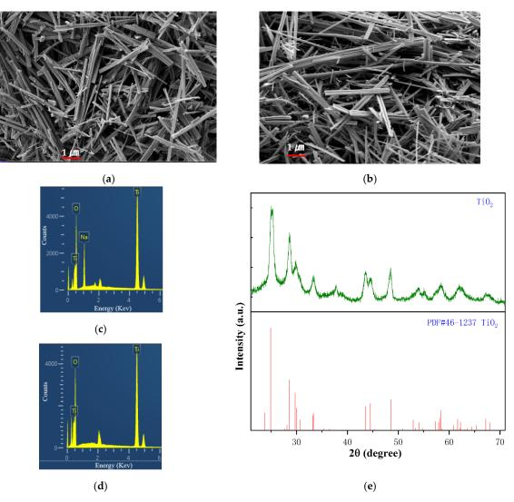
**Figure 1.** (a) SEM image of Na<sub>2</sub>TiO<sub>7</sub> nanobelt; (b) SEM image of TiO<sub>2</sub> nanobelt; (c,d) EDS spectra of TiO<sub>2</sub> and Na<sub>2</sub>Ti<sub>3</sub>O<sub>7</sub> nanobelt; (e) XRD patterns of TiO<sub>2</sub>. EDS, energy-dispersive X-ray spectroscopy.
