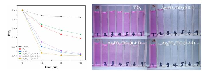
Figure 5. Photocatalytic degradation curves and images of Ag<sub>3</sub>PO<sub>4</sub>/TiO<sub>2</sub> composite.
