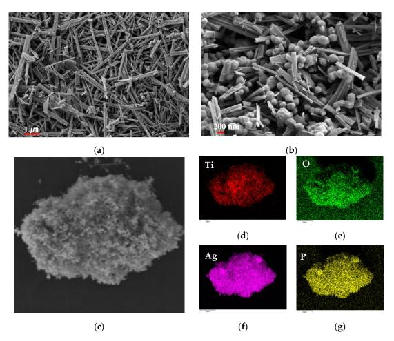
**Figure 4.** (**a**,**b**) SEM images of  $Ag_3PO_4/TiO_2$  composite; (**c**) The SEM image corresponding to map; (**d**) Map of Ti; (**e**) Map of O; (**f**) Map of Ag; (**g**) Map of P.
