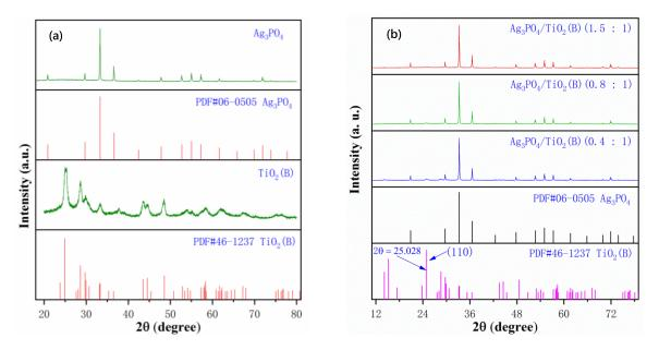
Figure 3. (a) XRD patterns of Ag<sub>3</sub>PO<sub>4</sub> and TiO<sub>2</sub>(B); (b) XRD patterns of Ag<sub>3</sub>PO<sub>4</sub>/TiO<sub>2</sub>(B) with different molar ratios.
