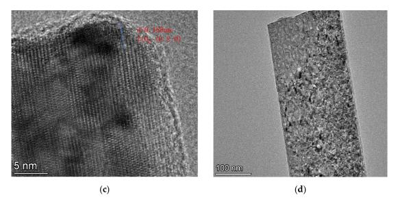
**Figure 2.** (**a**,**b**) Diffraction patterns of TiO<sub>2</sub>(B) nanobelt; (**c**,**d**) HRTEM (High-Resolution Transmission Electron Microscopy) images of TiO<sub>2</sub>(B) nanobelt.
