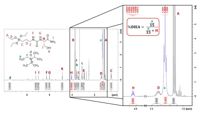
**Figure 2.** DIEA percentage calculation by  $^{1}$ H NMR (500 MHz, 25  $^{\circ}$ C). Example of Si-Ser-NH<sub>2</sub>. DIEA% was determined by using DIEA CH<sub>3</sub> signals (1.26–1.31 ppm) and amino amide CH $\alpha$  (4.01–4.26 ppm depending on amino amide).
