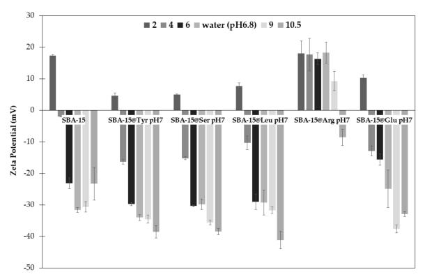
**Figure 11.** Zeta potential of bare SBA-15 and the SBA-15@AA samples as a function of pH. Measurements were performed at 25 °C and at a concentration of 0.24 mg/mL.
