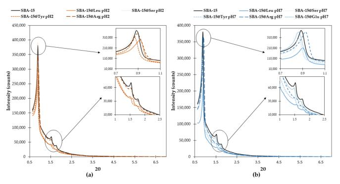
**Figure 8.** X-ray diffraction patterns of SBA-15 and functionalized SBA-15@AA obtained by acid catalysis (**a**) or nucleophilic catalysis at pH 7 (**b**).
