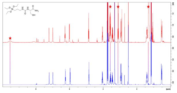
Figure 3. Comparison of <sup>1</sup>H NMR spectra of Si-Ser-NH<sub>2</sub> synthesized with DIEA (red) and sodium bicarbonate (blue).
