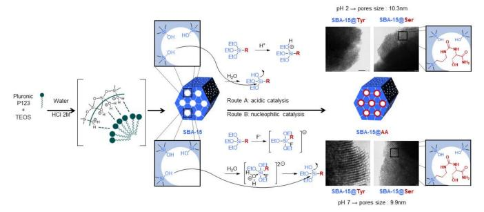
Figure 5. Schema of the SBA-15 functionalization with Si-AA-NH<sub>2</sub>.
