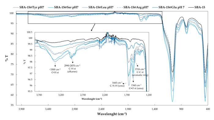
Figure 9. FT-IR spectra of the bare SBA-15 and the functionalized SBA-15@AA at pH 7.
