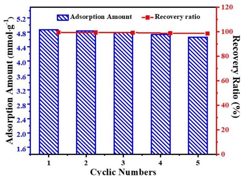
Figure 8. Cycling of CO<sub>2</sub> adsorption by GO(0.25)/MR-500 at 298.15 K and 500 kPa.
