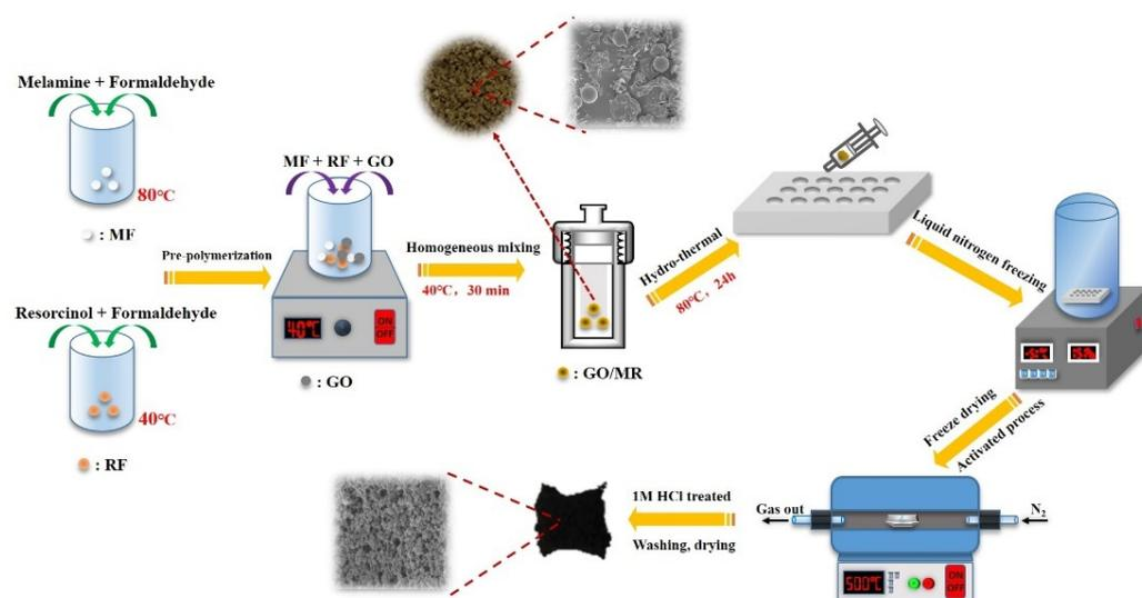
**Figure 1.** Schematic illustration of the synthesis process of nitrogen-rich porous carbon materials derived from GO/MR composite.
