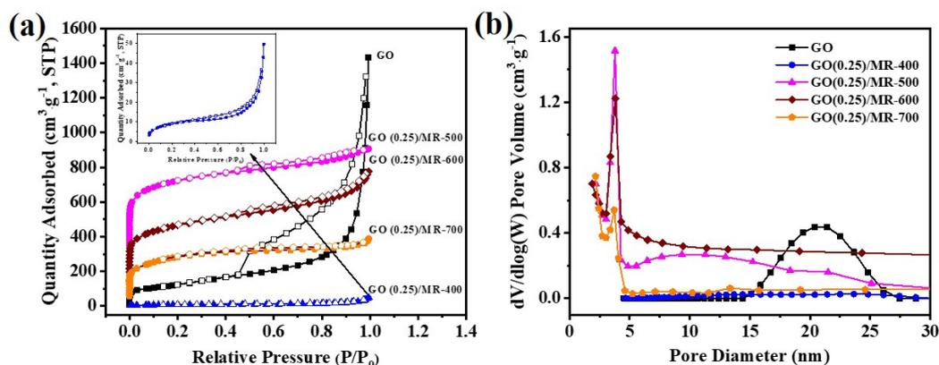
**Figure 2.** (a)  $\text{N}_2$  adsorption-desorption isotherms and (b) pore size distributions of GO and GO(0.25)/MR-derived nitrogen-rich porous carbon materials obtained at different activation temperature.
