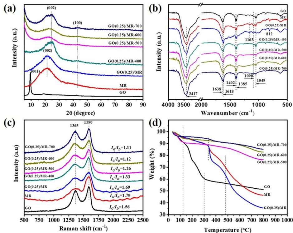
**Figure 4.** (a) XRD, (b) FTIR, (c) Raman patterns and (d) TGA curves of GO, MR, GO(0.25)/MR and GO(0.25)/MR-derived nitrogen-rich porous carbon materials obtained at different activation temperature.
