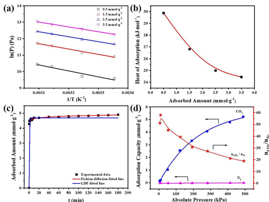
**Figure 7.** (a) Curves of  $\ln(P)$  versus  $(1/T)$ , (b) isosteric heat of adsorption at different  $\text{CO}_2$  adsorption capacities, (c)  $\text{CO}_2$  adsorption kinetics and (d) adsorption isotherms of  $\text{N}_2$  and  $\text{CO}_2$  at 298.15 K for GO(0.25)/MR-500.
