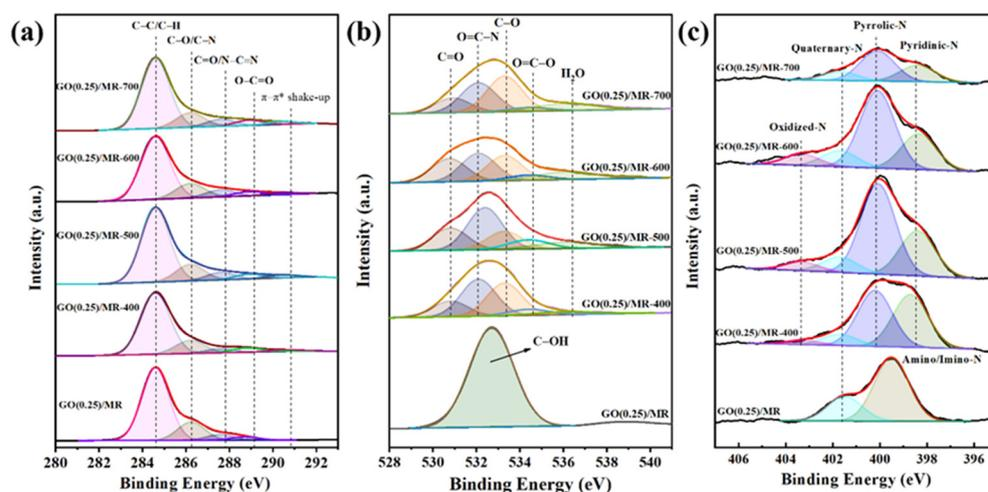
**Figure 5.** High resolution (a) C 1s, (b) O 1s and (c) N 1s XPS spectra of GO(0.25)/MR and GO(0.25)/MR-derived nitrogen-rich porous carbon materials obtained at different activation temperature.
