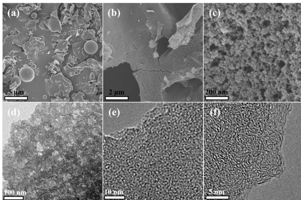
**Figure 3.** SEM images of (a) GO(0.25)/MR and (b,c) GO(0.25)/MR-500, (d) TEM image and (e,f) high-resolution TEM image of GO(0.25)/MR-500.
