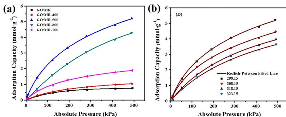
**Figure 6.** (a) CO<sub>2</sub> adsorption isotherms at 298.15 K for GO(0.25)/MR and GO(0.25)/MR-derived, nitrogen-rich porous carbon materials obtained at different activation temperature. (b) Redlich–Peterson isotherm models on experimental CO<sub>2</sub> adsorption at different temperature for GO(0.25)/MR-500.
