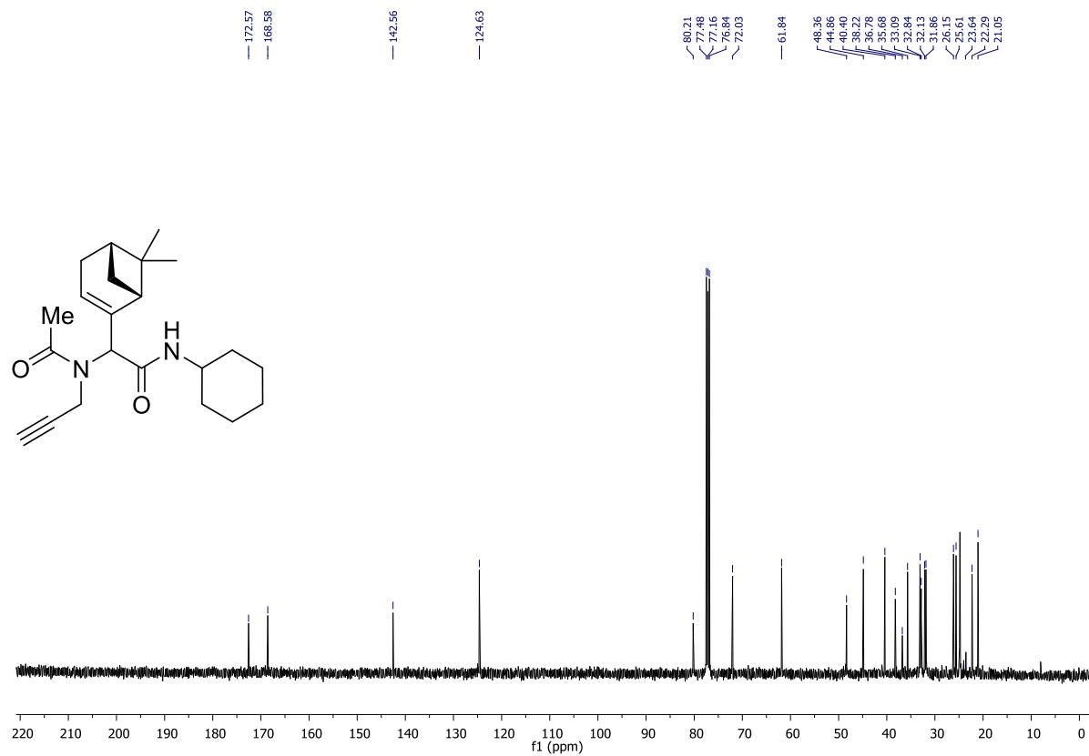
FIGURE S12. 100 MHz  $^{13}\text{C}$  NMR spectra in  $\text{CDCl}_3$  of major diastereomer of **1c**.
