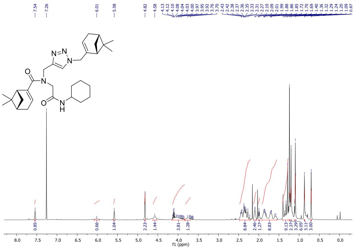
FIGURE S32. 400 MHz  $^1\text{H}$  NMR spectra in  $\text{CDCl}_3$  of **3d**.
