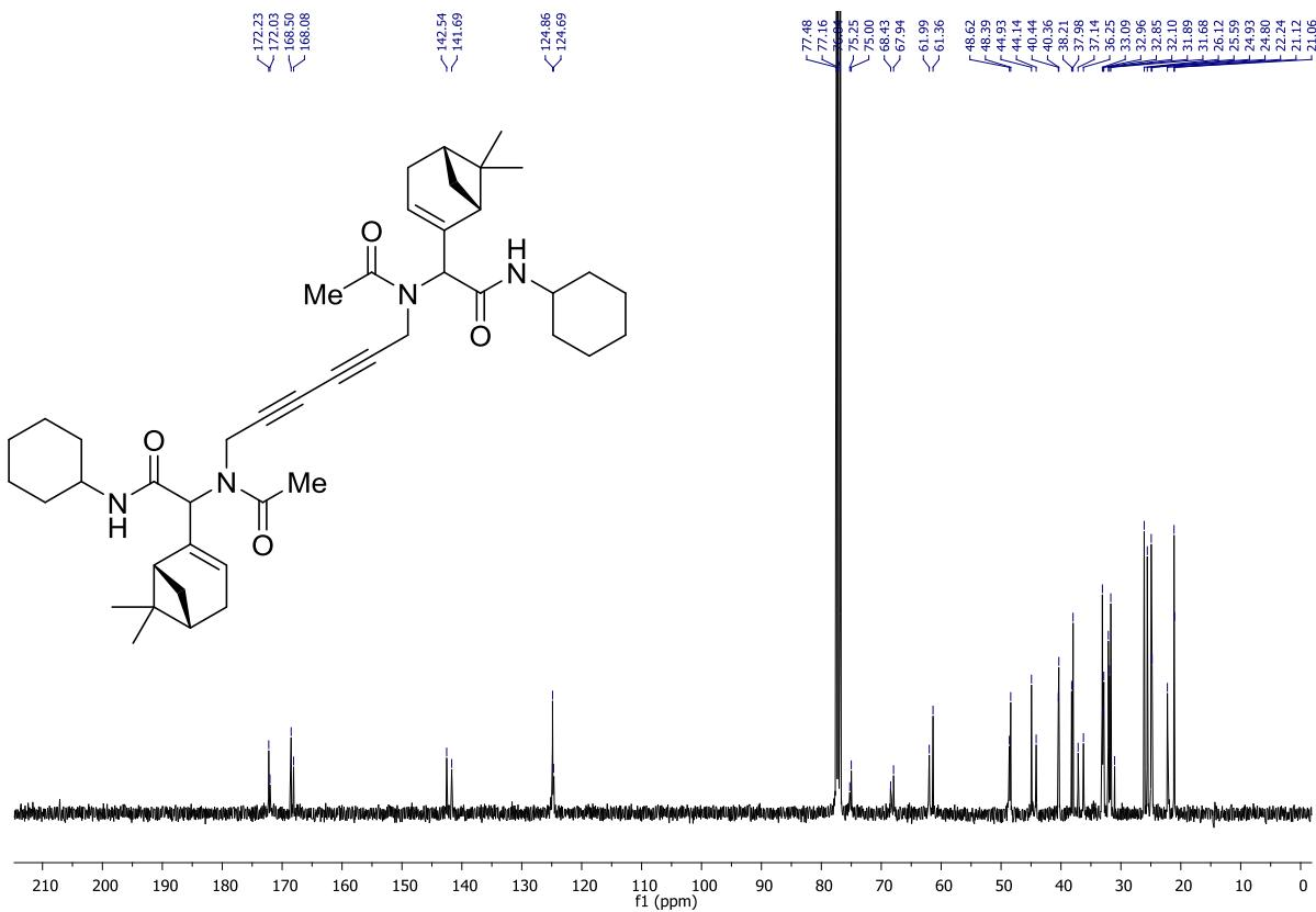
FIGURE S42. 100 MHz  $^{13}\text{C}$  NMR spectra in  $\text{CDCl}_3$  of **4b**.
