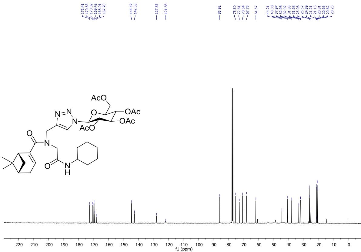
FIGURE S36. 100 MHz  $^{13}\text{C}$  NMR spectra in  $\text{CDCl}_3$  of **3e**.
