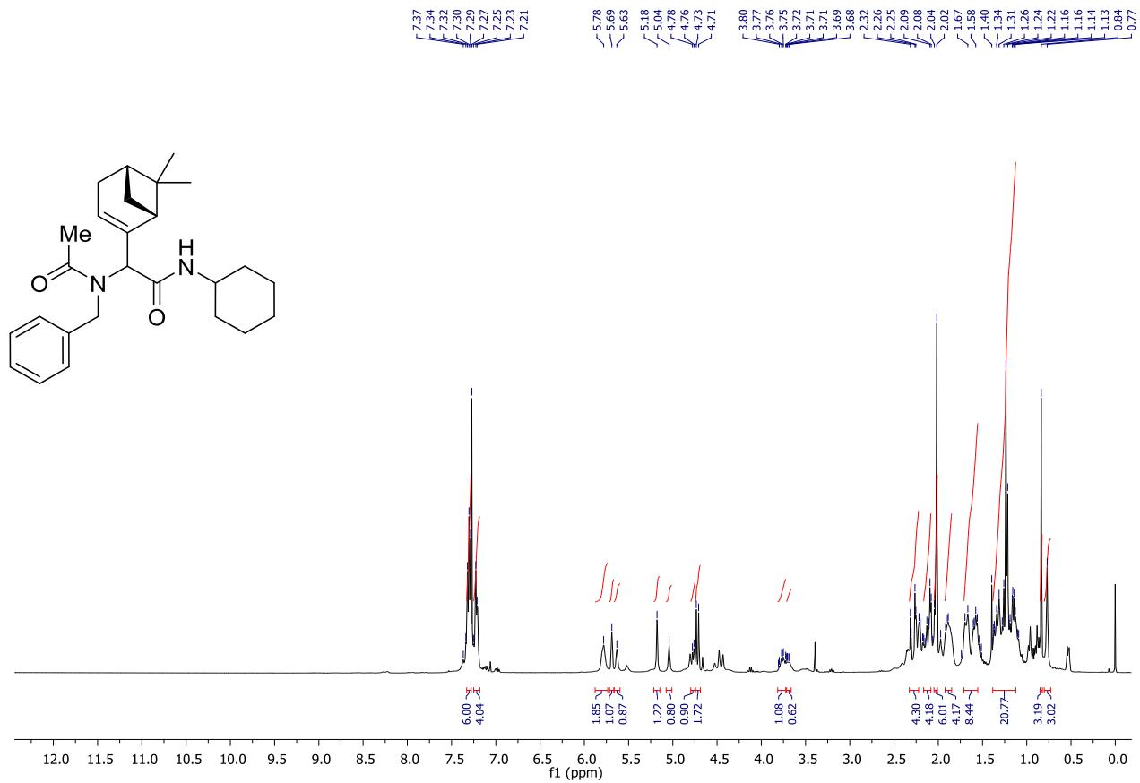
FIGURE S1. 400 MHz <sup>1</sup>H NMR spectra in CDCl<sub>3</sub> of **1a** (Crude mixture of diastereomers).
