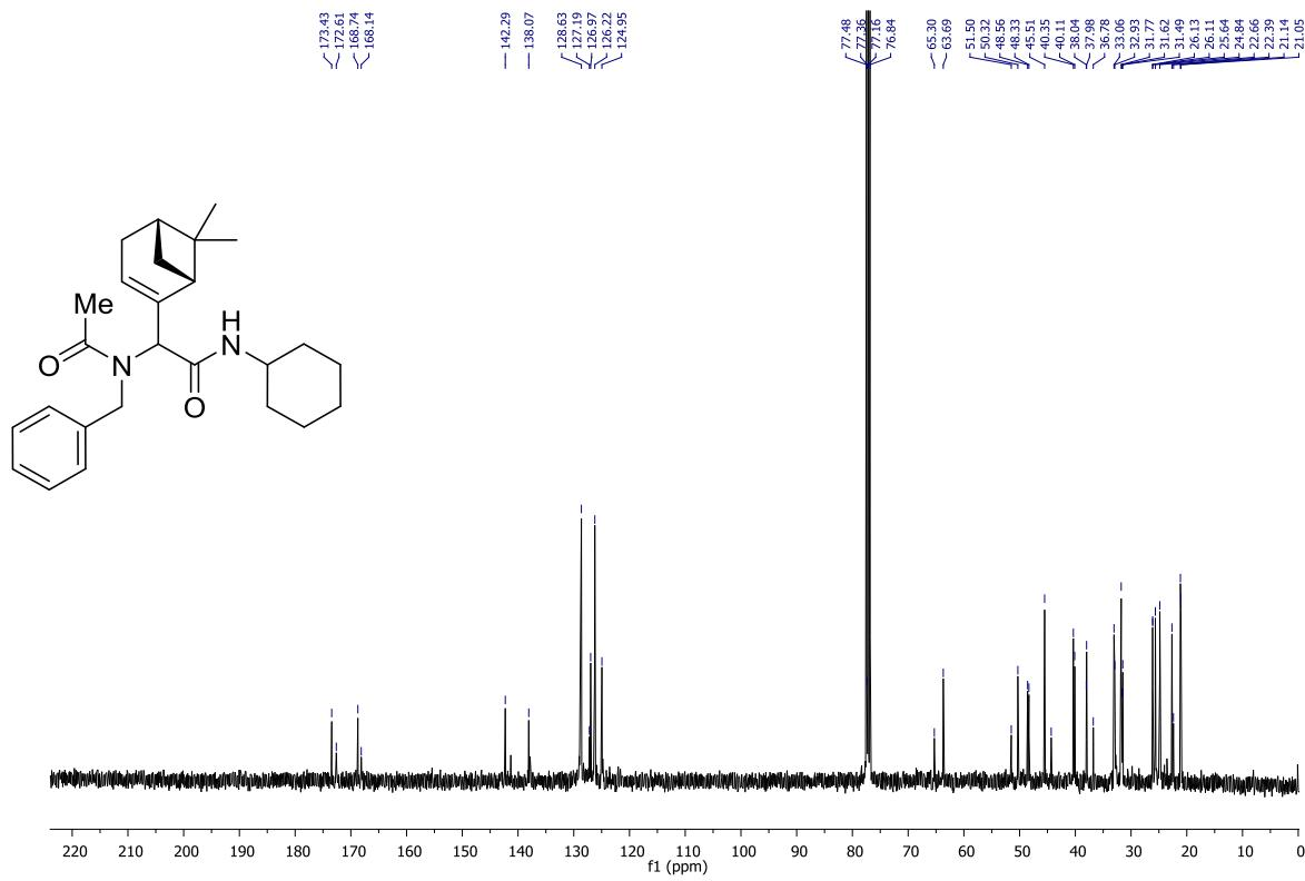
FIGURE S2. 100 MHz  $^{13}\text{C}$  NMR spectra in  $\text{CDCl}_3$  of **1a** (Crude mixture of diastereomers).
