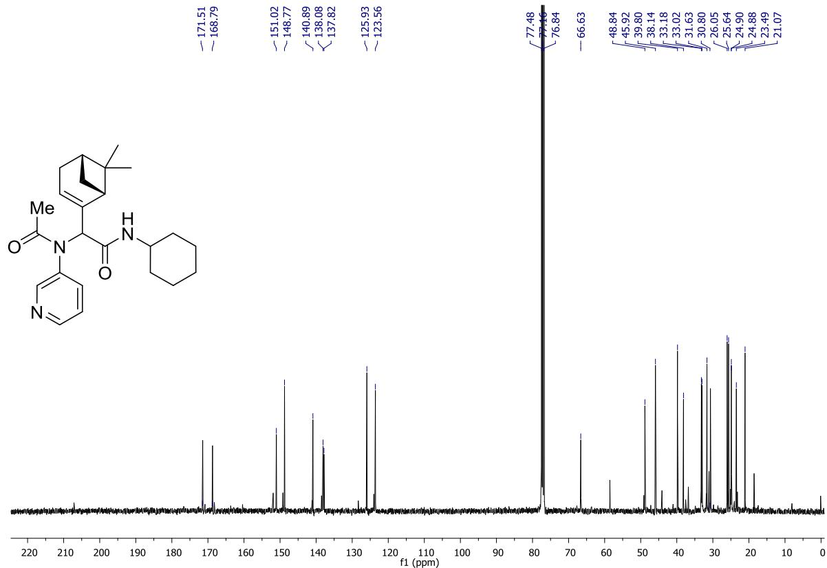
FIGURE S7. 100 MHz  $^{13}\text{C}$  NMR spectra in  $\text{CDCl}_3$  of **1b** (Crude mixture of diastereomers).
