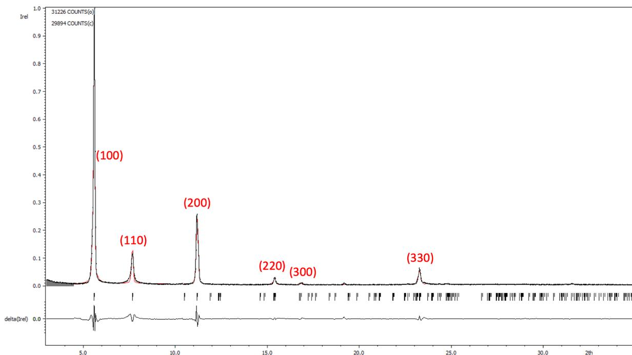
**Figure S4.** Diffraction pattern of the Phase-1: with  $P21/c$  space group (parameters listed in Table S2): experimental (black) and simulated (red).
