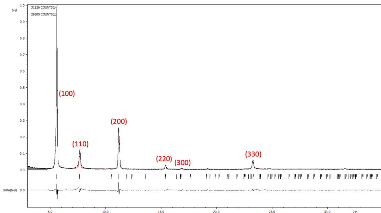
**Figure S3.** Diffraction pattern of the Phase-1 in *Pbcm* space group (parameters listed in Table S2): experimental (black) and simulated (red).
