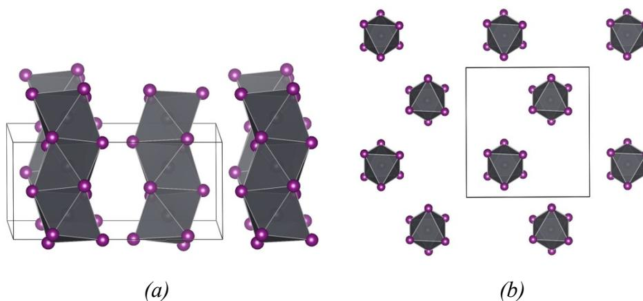
**Figure S5.** Probable crystal structure of Phase-1 (space group  $Pbcm$ ) with a single chains of  $PbI_6$  octahedra in  $yz$  (a) and  $xy$  (b) projections.
