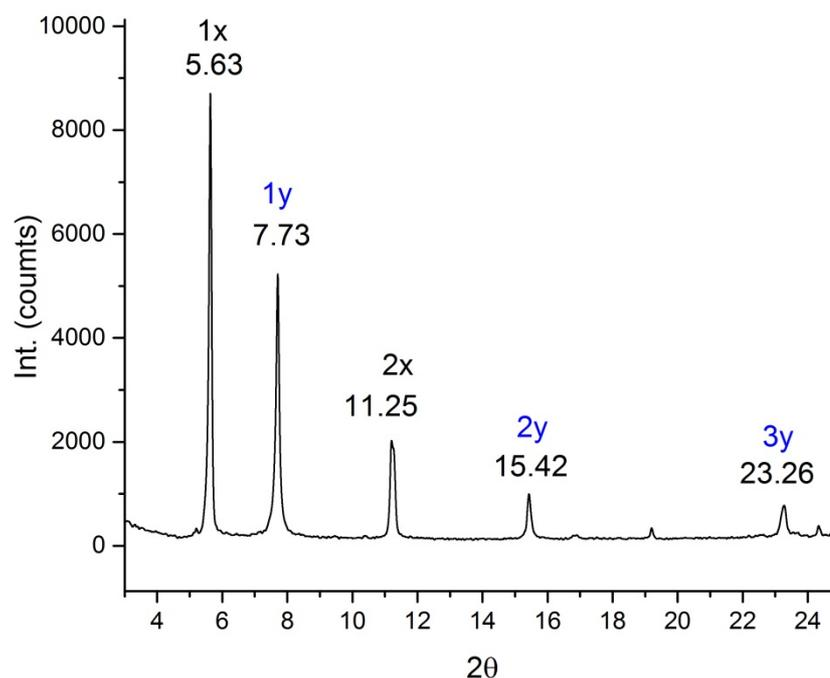
**Figure S2.** Diffraction pattern of the Phase-1 powder. The captions indicate the positions of reflections, symbols “x” and “y” indicate the affiliation for one of the two distinct groups of reflections.
