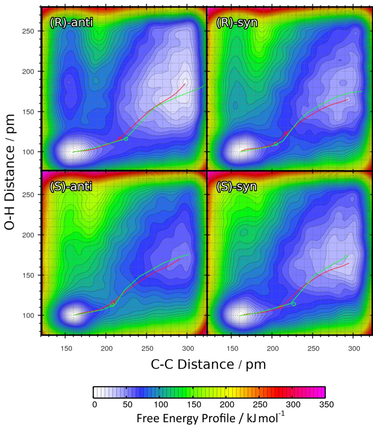
Figure S5: Free energy profiles of the Aldol reactions (R = iPr) in vacuum computed from HyAIMD Metadynamics; definition of collective variables see Figure 4. Red curves depict the minimum energy paths from educts (*upper-right basin*) to products (*lower-left basin*). Green curves show the results of static NEB calculations for comparison. Green circles denote the statically determined transition state.
