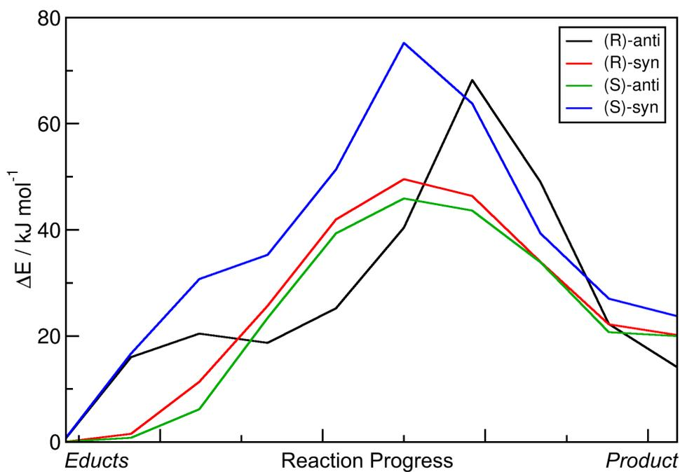
Figure S2: Energy profiles of Aldol reactions ( $R = iPr$ ) resulting from static NEB calculations. Energies are given relative to educts.
