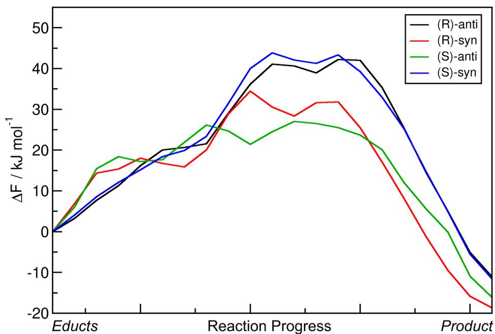
Figure S8: One-dimensional free energy profiles of Aldol reactions (R = Et) in DMF obtained from HyAIMD Metadynamics; corresponds to red curves in Figure S4.
