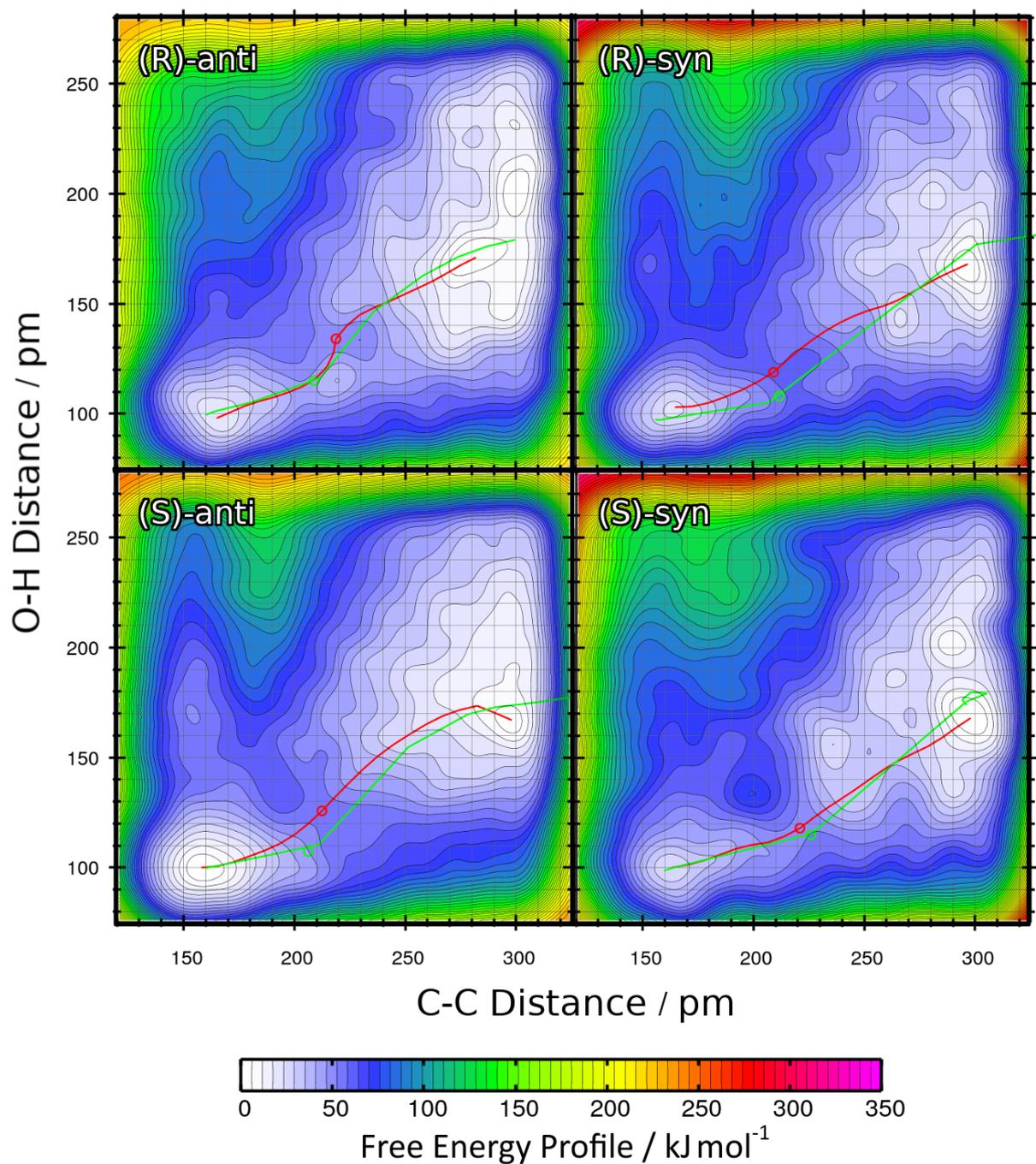
Figure S3: Free energy profiles of the Aldol reactions ( $R = Et$ ) in vacuum computed from HyAIMD Metadynamics; definition of collective variables see Figure 4. Red curves depict the minimum energy paths from educts (*upper-right basin*) to products (*lower-left basin*). Green curves show the results of static NEB calculations for comparison. Green circles denote the statically determined transition state.
