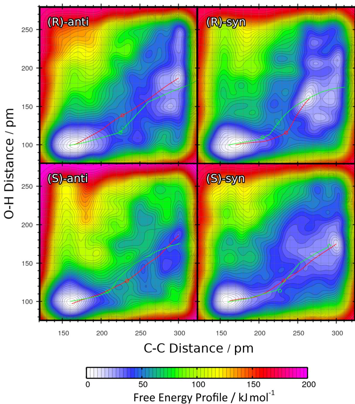
Figure S6: Free energy profiles of the Aldol reactions ( $R = iPr$ ) in DMF computed from HyAIMD Metadynamics; definition of collective variables see Figure 4. Red curves depict the minimum energy paths from educts (*upper-right basin*) to products (*lower-left basin*). Green curves show the results of static NEB calculations for comparison. Green circles denote the statically determined transition state.
