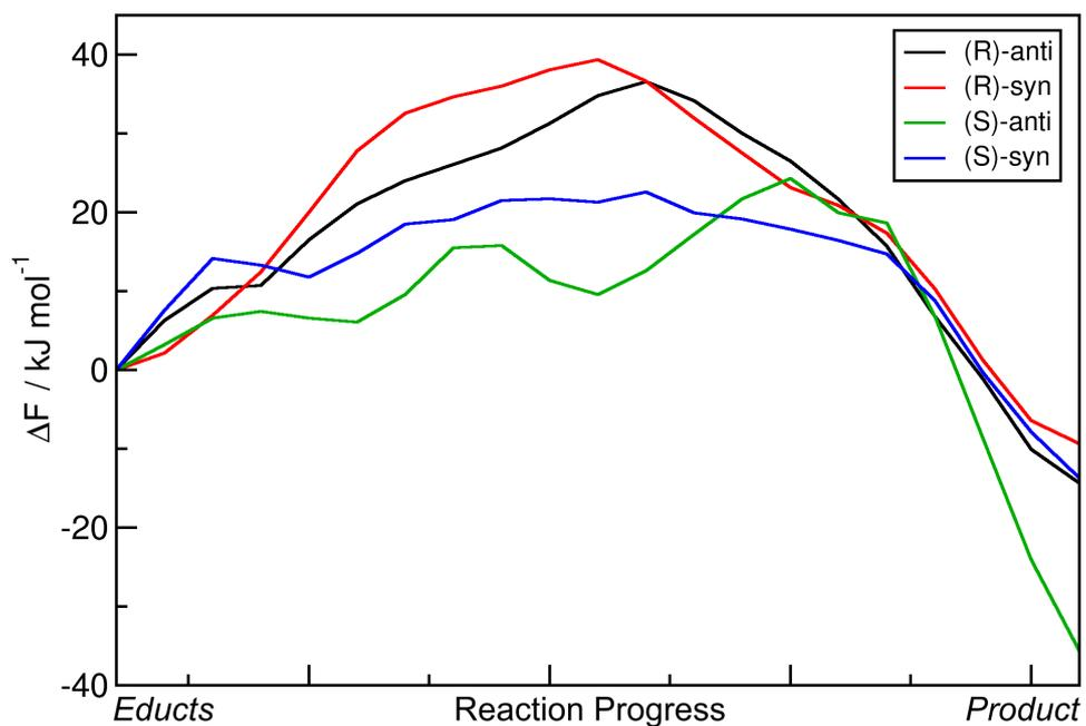
Figure S10: One-dimensional free energy profiles of Aldol reactions ( $R = iPr$ ) in DMF obtained from HyAIMD Metadynamics; corresponds to red curves in Figure S6.
