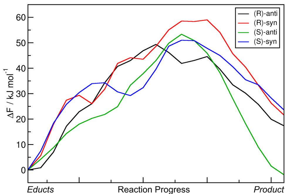
Figure S7: One-dimensional free energy profiles of Aldol reactions (R = Et) in vacuum obtained from HyAIMD Metadynamics; corresponds to red curves in Figure S3.
