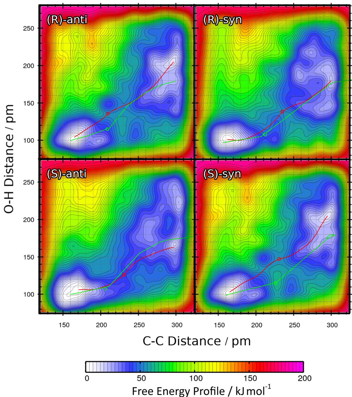
Figure S4: Free energy profiles of the Aldol reactions (R = Et) in DMF computed from HyAIMD Metadynamics; definition of collective variables see Figure 4. Red curves depict the minimum energy paths from educts (*upper-right basin*) to products (*lower-left basin*). Green curves show the results of static NEB calculations for comparison. Green circles denote the statically determined transition state.
