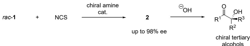
**Scheme 1.** Asymmetric construction of a tetrasubstituted stereogenic center by enantioselective decarboxylative chlorination and subsequent nucleophilic substitution.
