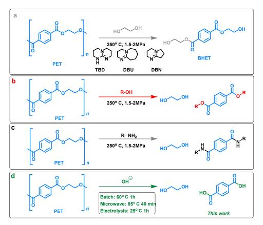
**Figure 1.** Chemical depolymerization methods for depolymerization of poly(ethylene terephthalate) (PET). (a) glycolysis (b) alcoholysis (c) aminolysis (d) chemical depolymerization methods in refluxing methanol and base in batch; at 85 °C in the microwave in 40 min; in an electrolysis experiment at room temperature.
