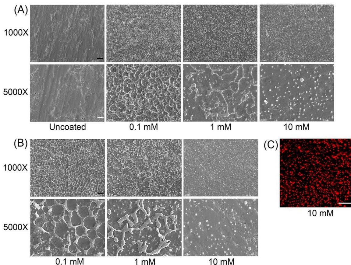
**Figure 1.** SEM (A,B) and fluorescence (C) images of phospholipid coats on Ti discs. Ti discs were coated with phospholipids by loading 0.1, 1, and 10 mM phospholipid solution, followed by drying and hydration for 6 (A) and 24 h (B). Black (A) and white (B) bars indicate 10 and 2 μm, respectively. White bar in (C) indicates 10 μm.
