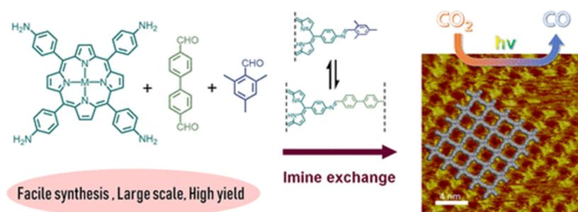
**Figure 2.** Schematic illustration of synthesis of the COF-367 NSs for  $\text{CO}_2$  photoreduction to CO and its STM image. Copied with permission from ACS 2020 [31].
