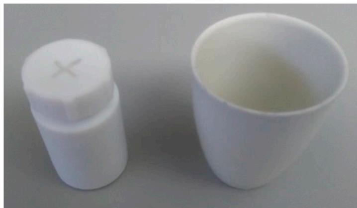
**Figure 24.** Polytetrafluoroethylene (PTFE) closed crucible and porcelain crucible respectively.
