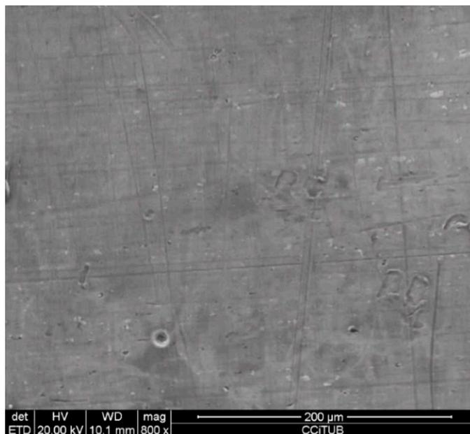
**Figure 2.** Detail of the aluminium specimen surface after 2000 h immersed in solar salt.
