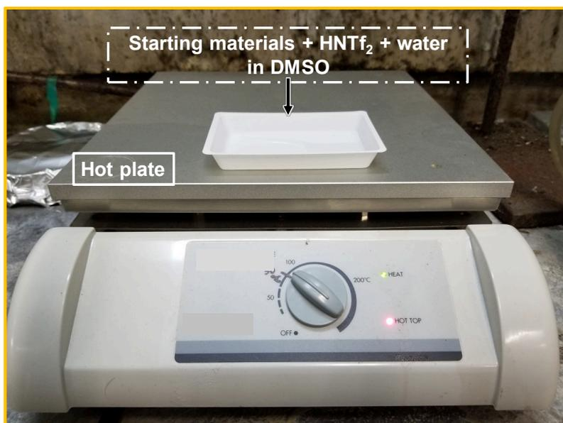
**Figure S14.** Photograph of the apparatus (hot plate), where the reactions were performed at *ca.* 60 °C.
