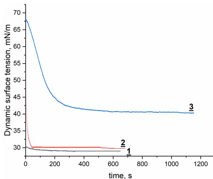
**Figure 2.** Dynamic surface tension for O-β-D-Galactopyranosyl-(1→4)-N-tetradecyl-(3-sulfopropyl)-D-glucosamine hydrochloride in concentrations: 1–30 mM, 2–0.3 mM, 3–0.0003 mM.
