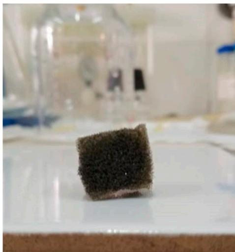
**Figure 8.** Image of the polyurethane-graphene oxide (PU-GO) sponge.
