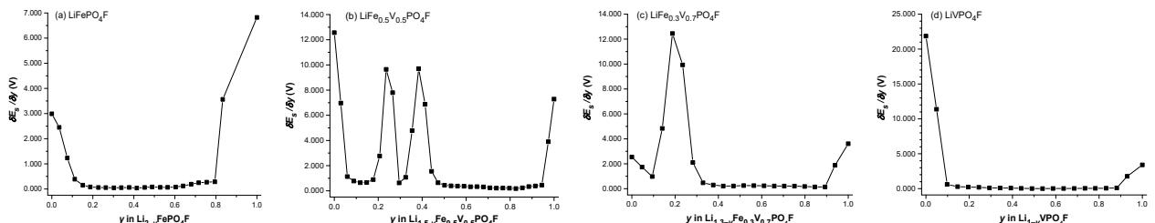
**Figure S6.** Plots of the slope of quasi-equilibrium OCVs as a function of  $\text{Li}^+$ -extraction content  $y$  ( $\delta E_s / \delta y$ ) and the fitted lines in  $\text{Li}_{1-y}\text{Fe}^{\text{III}}_{1-x}\text{V}_x\text{PO}_4\text{F}$ , *i.e.*  $\text{Li}_{2-x-y}\text{Fe}^{\text{II}}_{1-x}\text{V}_x\text{PO}_4\text{F}$  with  $x = 0$  (a),  $x = 0.5$  (b),  $x = 0.7$  (c) and  $x = 1$  (d).
