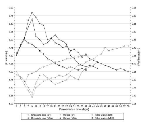
Figure 2. Variation in pH and VFA/TA during anaerobic digestion process of CB, W, and FW.
