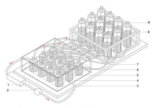
**Figure 1.** Biofermenter for biogas production tests (18-chamber section): 1—water heater with temperature adjustment; 2—water pump; 3—insulated tubes for liquid heating medium; 4—water jacket (39 °C); 5—biofermenter (1.4 dm<sup>3</sup>); 6—slurry-sample drawing tube; 7—tube for transporting the biogas; 8—graduated tank for biogas; 9—gas sampling valve.
