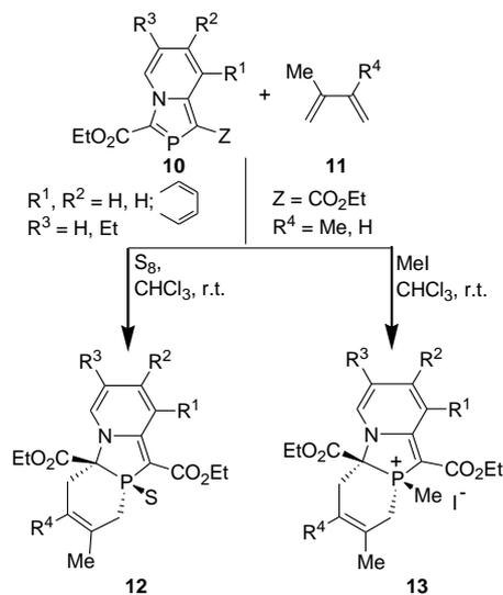
**Scheme 5.** DA reactions of 1,3-bis(ethoxycarbonyl)-1,3-azaphospholo[5,1-*a*]pyridines with 2,3-dimethyl-1,3-butadiene (DMB) and isoprene.
