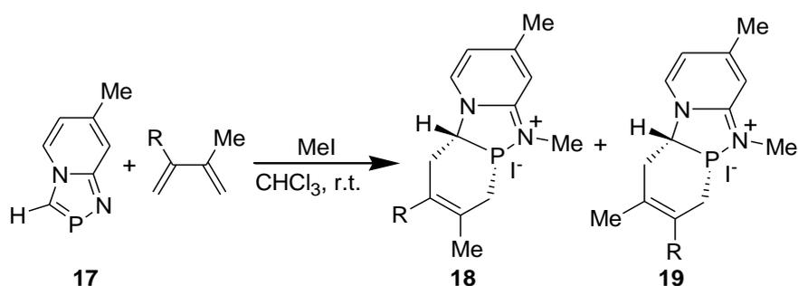
**Scheme 7.** DA reaction of 7-methyl-1,4,2-diazaphospholo[4,5-*a*]pyridine in the presence of methyl iodide.
