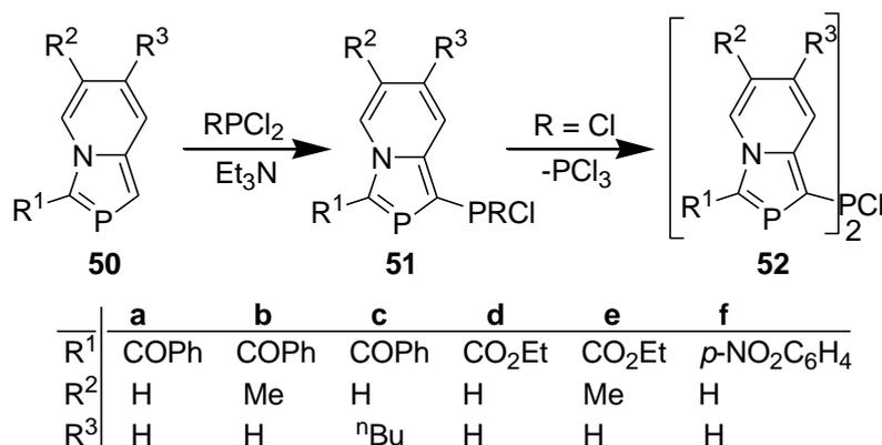
**Scheme 14.** Reaction of 1-unsubstituted 2-phosphaindolizines with chlorophosphines.
