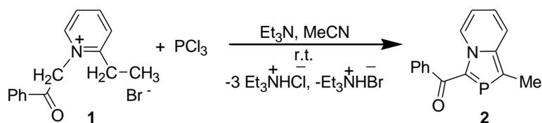
Scheme 1. Synthesis of 2-phosphaindolizine derivative.
