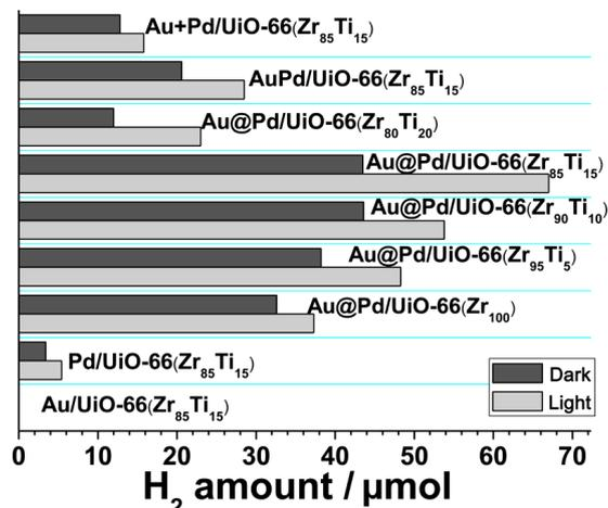
**Figure 5.** Amount of H<sub>2</sub> produced through formic acid dehydrogenation in the dark (black bars) or under visible light irradiation (gray bars,  $\lambda > 420$  nm,  $320 \text{ mW}\cdot\text{cm}^{-2}$ ) over different catalysts. Reproduced with permission from Reference [91]. Copyright 2017, American Chemical Society.
