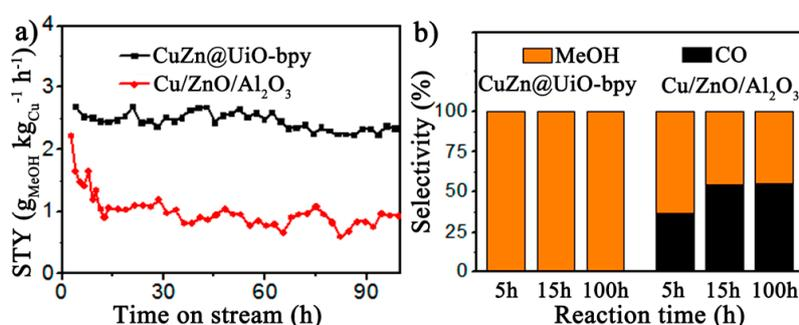
**Figure 2.** (a) The space-time yield (STY) of MeOH vs reaction time over a period of 100 h on stream; (b) Selectivity of product vs reaction time. Reproduced with permission from Reference [55]. Copyright 2017, American Chemical Society.
