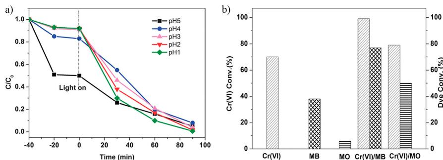
**Figure 9.** (a) Photocatalytic reduction of aqueous hexavalent chromium (Cr(VI)) with different amounts of H<sub>2</sub>SO<sub>4</sub> solution (0.2 M); and (b) Simultaneous photocatalytic reduction of Cr(VI) and degradation of dyes (10 ppm) over Pd@UiO-66-NH<sub>2</sub> under visible light irradiation ( $\lambda \geq 420$  nm). Reproduced with permission from Reference [155]. Copyright 2013, The Royal Society of Chemistry.
