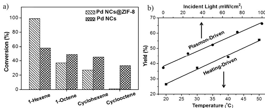
**Figure 7.** (a) Conversions of the hydrogenation of various alkenes over Pd NCs@ZIF-8 and Pd NCs under  $100 \text{ mWcm}^{-2}$  full-spectrum irradiation at room temperature; (b) The yields of the hydrogenation of 1-hexene with 1atm  $\text{H}_2$  over Pd NCs@ZIF-8 under full-spectrum irradiation with different light intensities at room temperature or upon heating at different temperatures. Reproduced with permission from Reference [24]. Copyright 2016, John Wiley & Sons, Inc.
