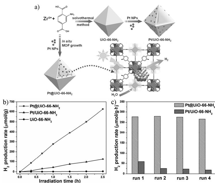
**Figure 6.** (a) Schematic illustration for the synthesis of Pt@UiO-66-NH<sub>2</sub> and Pt/UiO-66-NH<sub>2</sub>; (b) The photocatalytic hydrogen-production rates of UiO-66-NH<sub>2</sub>, Pt@UiO-66-NH<sub>2</sub>, and Pt/UiO-66-NH<sub>2</sub>; and, (c) Recycling performance comparison between Pt@UiO-66-NH<sub>2</sub> and Pt/UiO-66-NH<sub>2</sub>. Reproduced with permission from Reference [36]. Copyright 2016, John Wiley & Sons, Inc.
