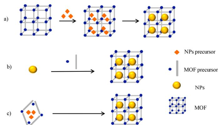
**Figure 1.** Main approaches for the fabrication of nanoparticle/MOF composites. (a) Ship in bottle; (b) bottle around ship; and, (c) in situ one-step synthesis.
