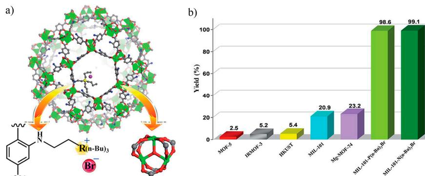
**Figure 4.** (a) The structure of the catalysts MIL-101-N(*n*-Bu)<sub>3</sub>Br and MIL-101-P(*n*-Bu)<sub>3</sub>Br (Cr: green; C: gray; O: red; N: blue; Br: amaranth, and R=N or P); (b) The yield of PC from the cycloaddition of PO and CO<sub>2</sub> catalyzed by different MOF catalysts. Reproduced with permission from Reference [72]. Copyright 2015, The Royal Society of Chemistry.
