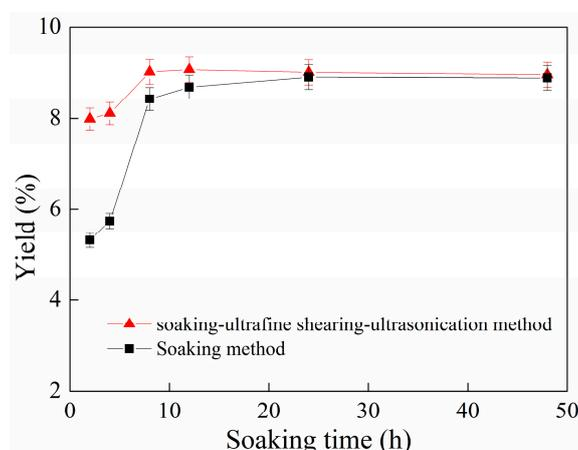
**Figure 6.** Relationship of soaking time and yield of C-PC based on the method of soaking-ultrafine shearing-ultrasonication. Error bars indicate standard deviations of the means ( $n = 3$ ).
