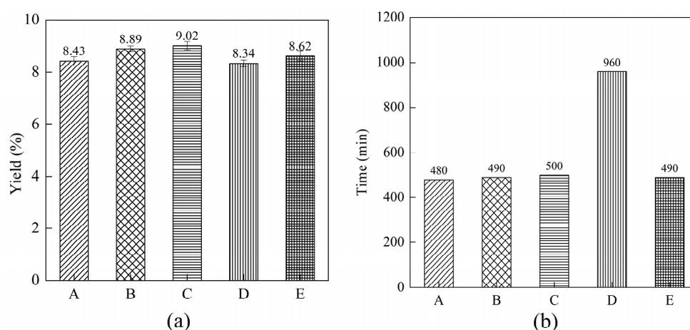
**Figure 7.** Comparison of the different cell disruption methods. Error bars indicate standard deviations of the means ( $n = 3$ ): (a) the yield of C-PC; (b) the extraction time.
