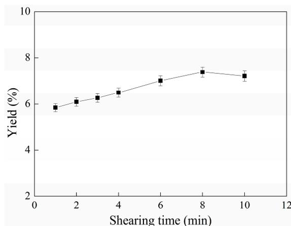
**Figure 2.** Relationship between shearing time and yield of C-PC. Error bars indicate standard deviations of the means ( $n = 3$ ).
