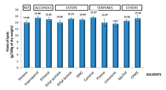
**Figure 2.** Comparison of yields obtained by several solvents to determinate the best solvent for the extraction of yeast oil.
