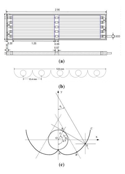
**Figure 13.** Solar CPC Photoreactor details: (a) superior and lateral views and (b) frontal view showing the curvature of the compound parabolic collectors; (c) CPC involute design.
