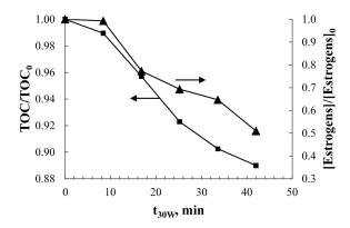
**Figure 2.** Solar photolytic degradation (**right axis**) and mineralization (**left axis**) of the commercial formulation of E2 and nomegestrol acetate mixture with an initial concentration of 5 ppm of estrogens and 388 ppm of TOC at pH 4.5 and with 97.2 kJ/m<sup>2</sup> of accumulated solar radiation (measured as UV-A).
