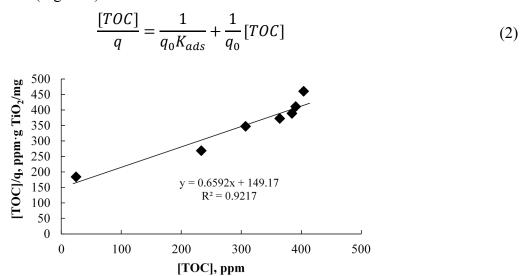
**Figure 4.** Linear regression of the Langmuir isotherm obtained from experiments at 30 °C, pH 6.9 and with 0.6 g/L of catalyst load.
