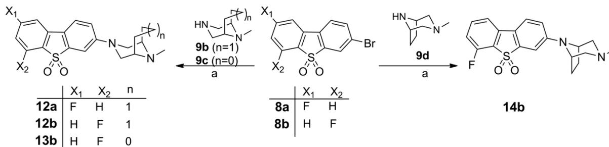
**Scheme 4.** Synthesis of the fluorinated reference compounds **12a,b**, **13b**, and **14b**. Reagents and conditions: (a) Pd<sub>2</sub>(dba)<sub>3</sub>, BINAP, Cs<sub>2</sub>CO<sub>3</sub>, toluene, 90 °C, 24–36 h, 38% for **12a**, 42% for **12b**, 47% for **13b**, and 67% for **14b**.
