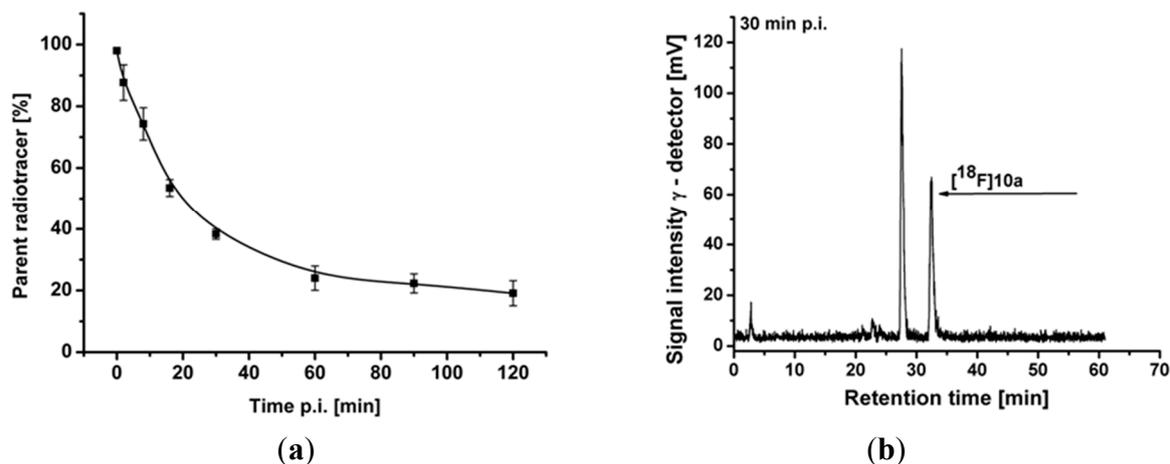
**Figure 4.** (a) Tri-exponential function fitting of the percentage of [ $^{18}\text{F}$ ]**10a** under baseline conditions ( $n = 3$ ) which was used to obtain metabolite-corrected arterial plasma input functions for modelling; (b) Representative radio-chromatogram of a pig plasma sample obtained at 30 min after intravenous injection of [ $^{18}\text{F}$ ]**10a** under baseline conditions.
