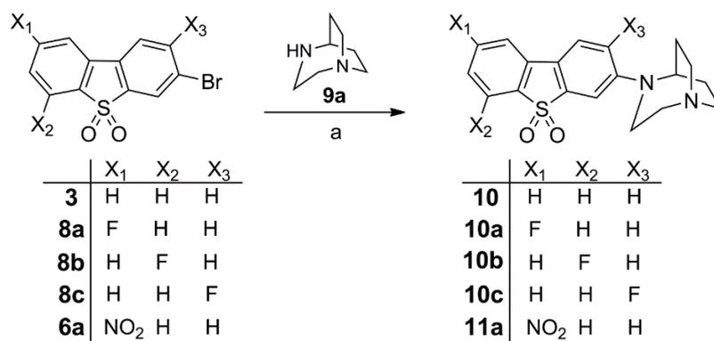
**Scheme 3.** Synthesis of **10**, fluorinated reference compounds **10a–c**, and nitro precursor **11**. Reagents and conditions: (a) Pd<sub>2</sub>(dba)<sub>3</sub>, BINAP, Cs<sub>2</sub>CO<sub>3</sub>, toluene, 90 °C, 24–36 h, 52% for **10a**, 48% for **10b**, 44% for **10c**, 73% for **10**, and 53% for **11a**.
