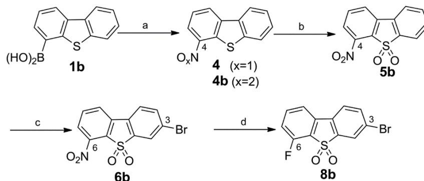
**Scheme 2.** Synthesis of 3-bromo dibenzothiophene intermediates **6b** and **8b**. Reagents and conditions: (a) *tert*-butyl nitrite, MeCN, 55 °C, 24 h, mixture of **4/4b** (~88:12); (b)  $\text{H}_2\text{O}_2$  (50%), HOAc, 120 °C, 5 h, 72% (two steps); (c) NBS, conc.  $\text{H}_2\text{SO}_4$ , r.t., 24 h, 78%; (d) TMAF·4 $\text{H}_2\text{O}$ , cyclohexane/DMSO, 6 h (azeotropic drying with separation of  $\text{H}_2\text{O}$ ), compound **6b**, 95 °C, 5 h, 73%.
