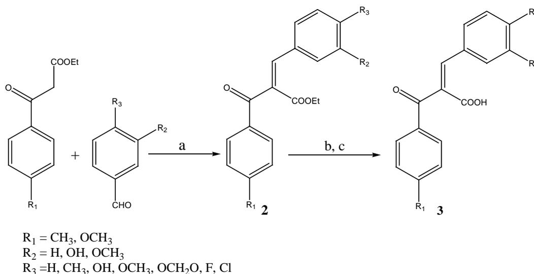
*Reagents and conditions:* (a)  $\text{CH}_3\text{COOH}$ ,  $\text{H}_2\text{N}(\text{CH}_2)_5\text{COOH}$ , PhMe, reflux; (b) 6 N NaOH, EtOH, r.t.; (c) 6 N HCl.
