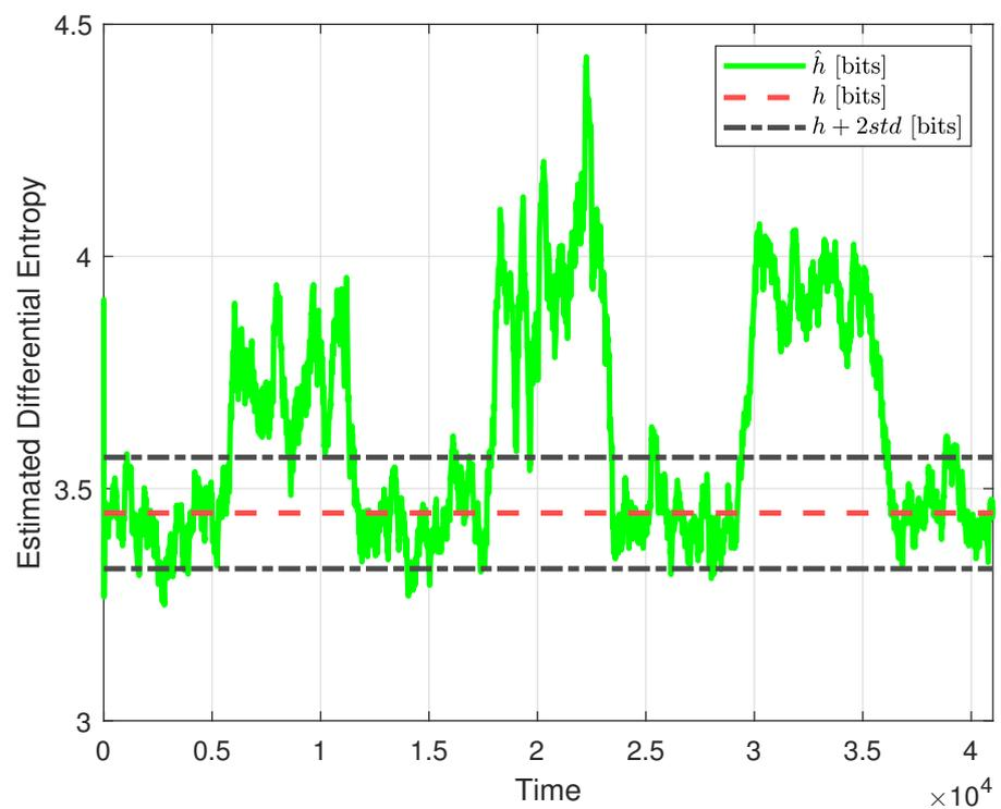
**Figure 5.** Estimated differential entropy of the signal  $u(k)$ , when faults in (21) and (22) are present, for the selected value of  $L = 300$  (green solid line), no-fault theoretical value (red dashed line), and no-fault theoretical value plus two standard deviations (black dash-dotted lines).
