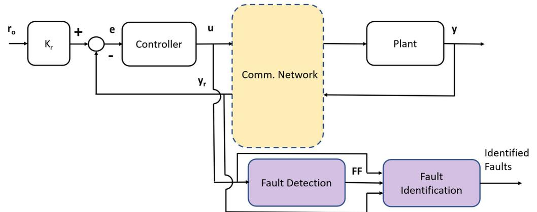
**Figure 1.** NCS SISO feedback loop with residual generator and fault-detection stages.
