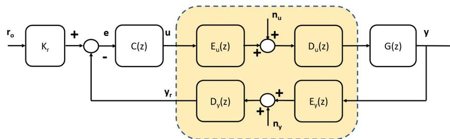
**Figure 2.** NCS SISO feedback loop with an AWGN network.
