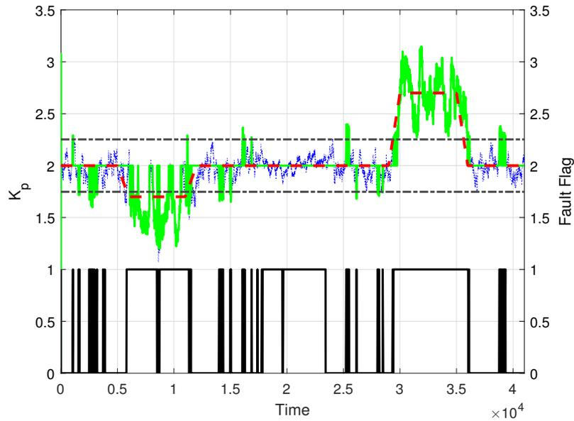
**Figure 6.** Estimated value of the plant gain parameter  $K_p$  for the selected value of  $L = 300$  (green solid line), true parameter value (red dashed line), standard deviation  $\sigma_{k_p}$  (black dash-dotted line), and reported fault flag (black solid line at the bottom).
