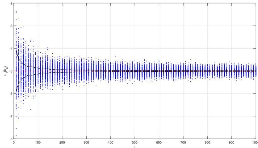
**Figure 3.** Monte Carlo simulation of  $u_1(k_o)$  as a function of  $L$  for  $k_o = 3000$  (blue dots), predicted mean value  $\mu_u$  (red dashed line), and variance of  $u_1(k_o)$  as a function of  $L$  (black dash-dotted line).
