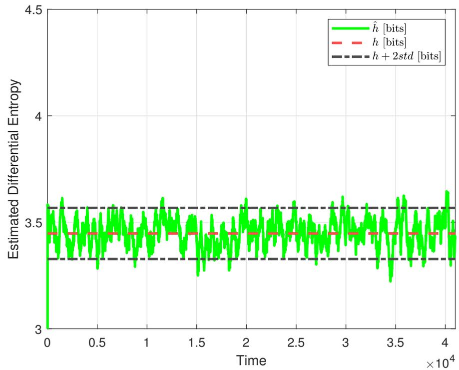
**Figure 4.** Estimated differential entropy of the signal  $u(k)$ , when no faults are present, for the selected value of  $L = 300$  (green solid line), no-fault theoretical value (red dashed line), and no-fault theoretical value plus two standard deviations (black dash-dotted lines).
