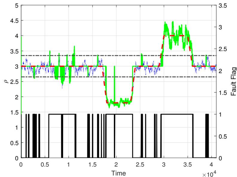
**Figure 7.** Estimated value of the plant gain parameter,  $\rho$ , for the selected value of  $L = 300$  (green solid line), true parameter value (red dashed line), standard deviation  $\sigma_\rho$  (black dash-dotted line), and reported fault flag (black solid line at the bottom).
