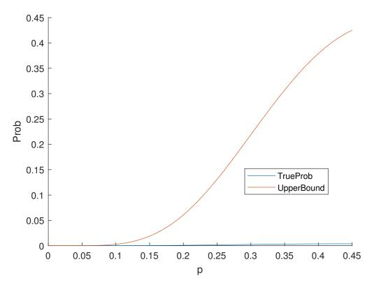
Figure 2. The Probability of Undetected Error of the Nordstrom-Robinson Code.
